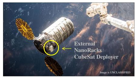
A robotic arm prepares to grapple an Orbital ATK Cygnus commercial re-supply spacecraft upon arrival at the International Space Station. The National Reconnaissance Office's OA-8 CubeSats were launched and deployed from an external NanoRacks CubeSat deployer, attached to the exterior of a Cygnus spacecraft.
