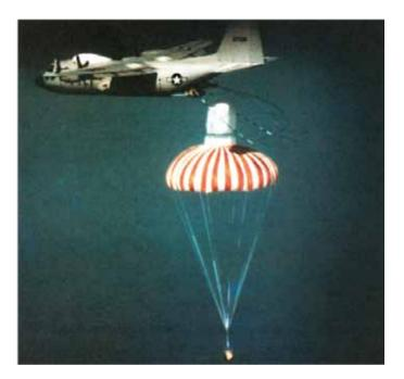
Figure 3. Aerial Recovery of Hexagon Film by JC-130 Aircraft (Reprinted from Oder, et. al., 1992, p. 98).
