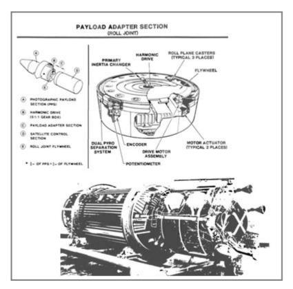
Figure 2. Gambit-3 Roll Joint and Aft Section of Spacecraft (reprinted from Oder, et. al., 1991, p. 57 and 82).
