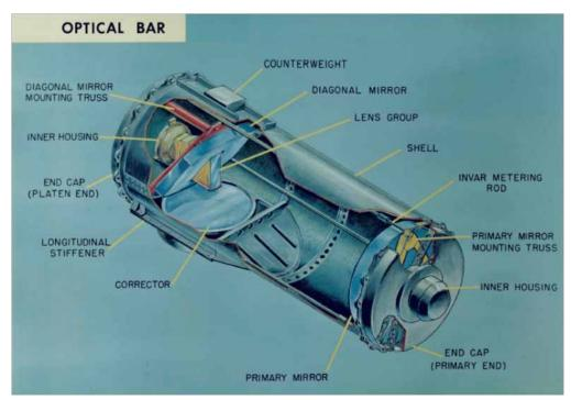
Figure 7. Hexagon Optical Bar.
