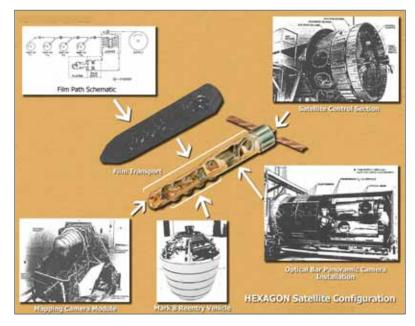
**Figure 4.** Hexagon Satellite Configuration (Figures 3 and 4 compiled from separate figures in Oder, et. al., 1992).
