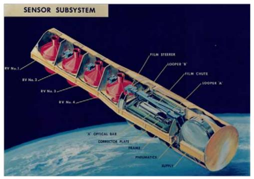
Figure 6. Hexagon Sensor Subsystem.
