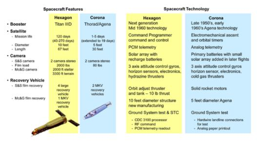
Figure 2. Hexagon-Corona Comparison (Graphic Courtesy of Lockheed-Martin Corp.)
