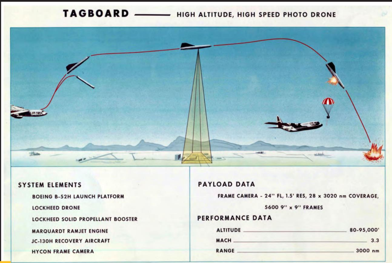
▶ Diagram of D-21 Drone (Codename TAGBOARD).
