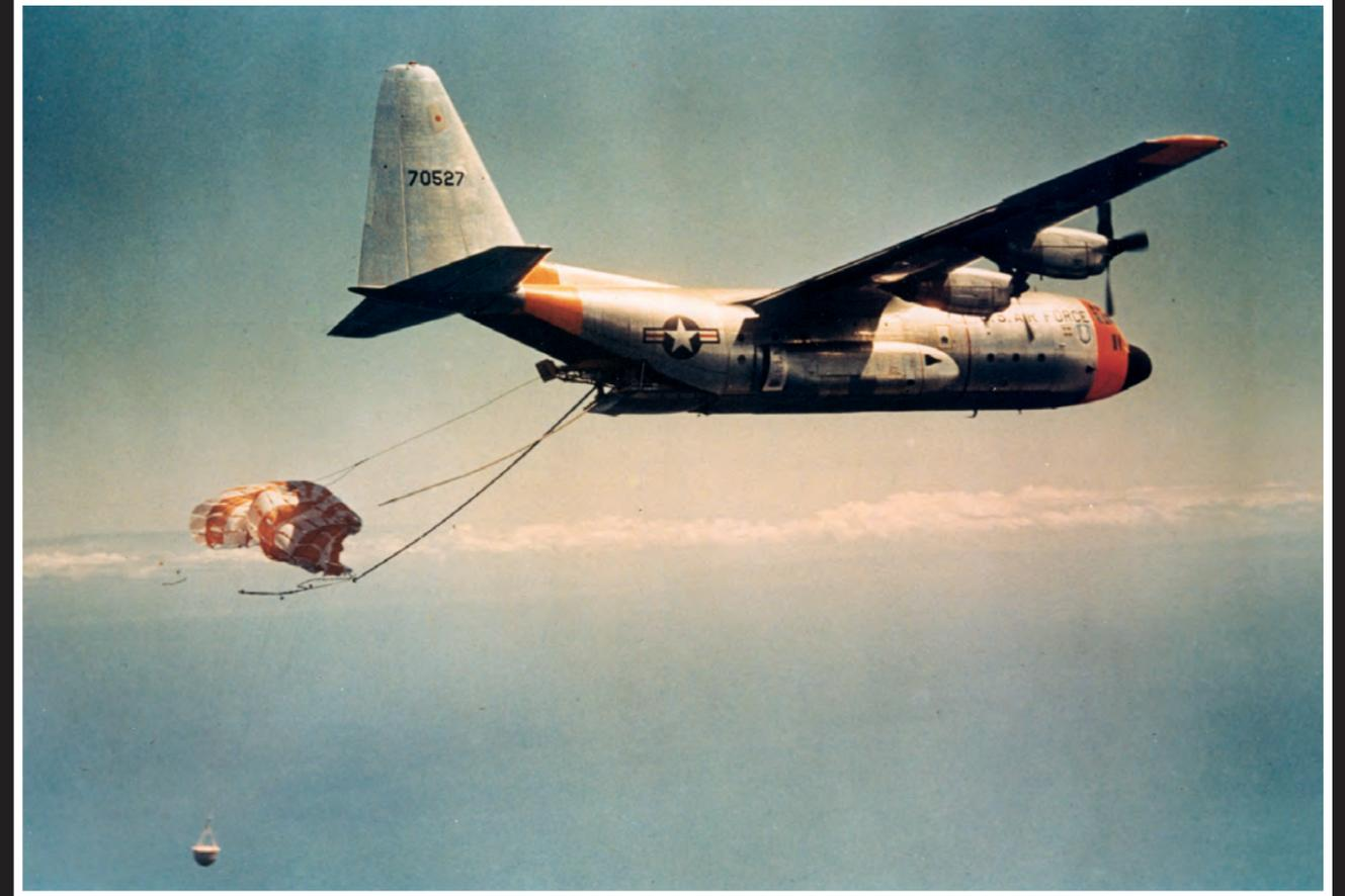
C-130 aircraft recovering parachute with Gambit satellite payload. ◀
