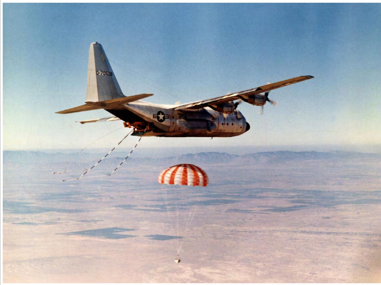
▶ JC-130 aircraft recovering parachute with test payload.
