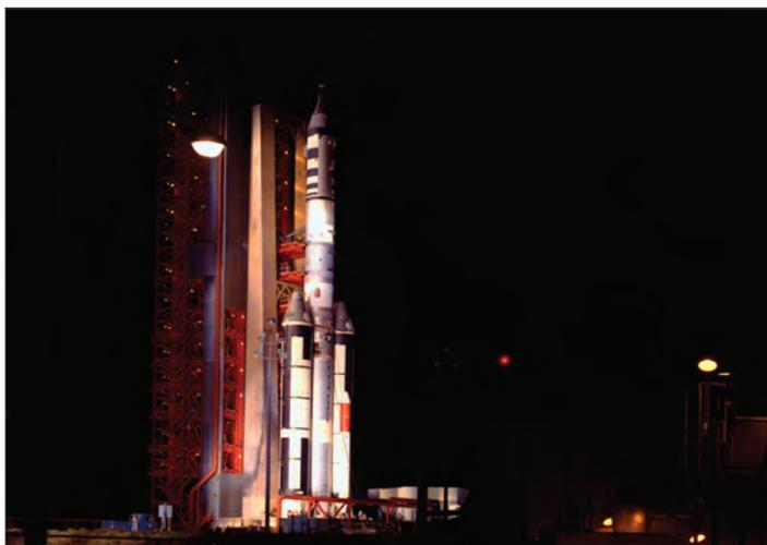
▲ An illuminated launch pad, against the November 1966 night sky, captures the MOL prepared for an unmanned flight to test the ablative shield.
