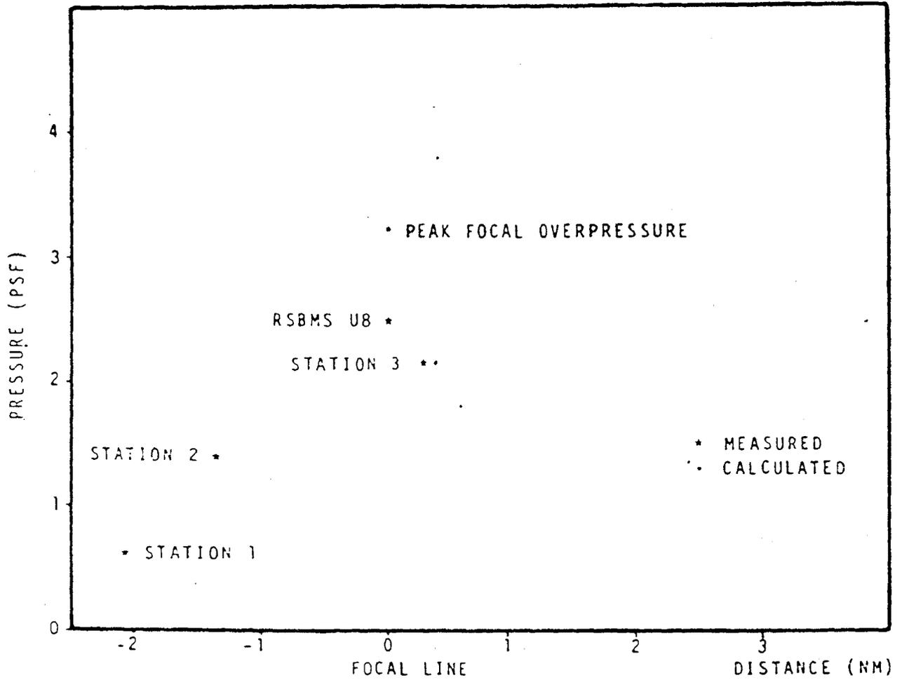
Figure 3-5. Sonic Boom Near Focus Line (Predicted vs Measured) STS-41D
