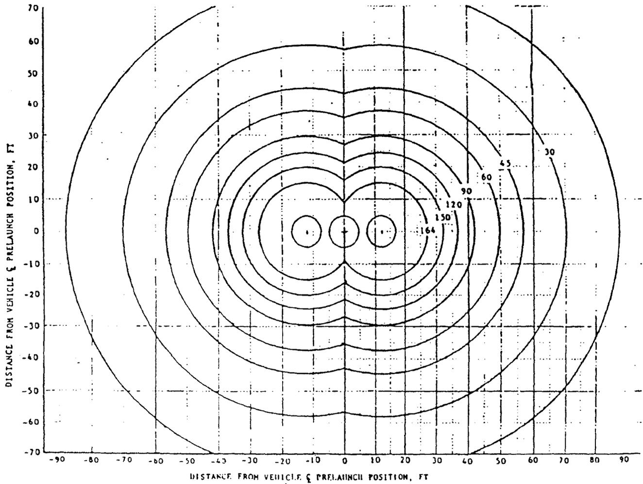
Figure 2-11. Dispersed Isobars of Max Splash Pressure
