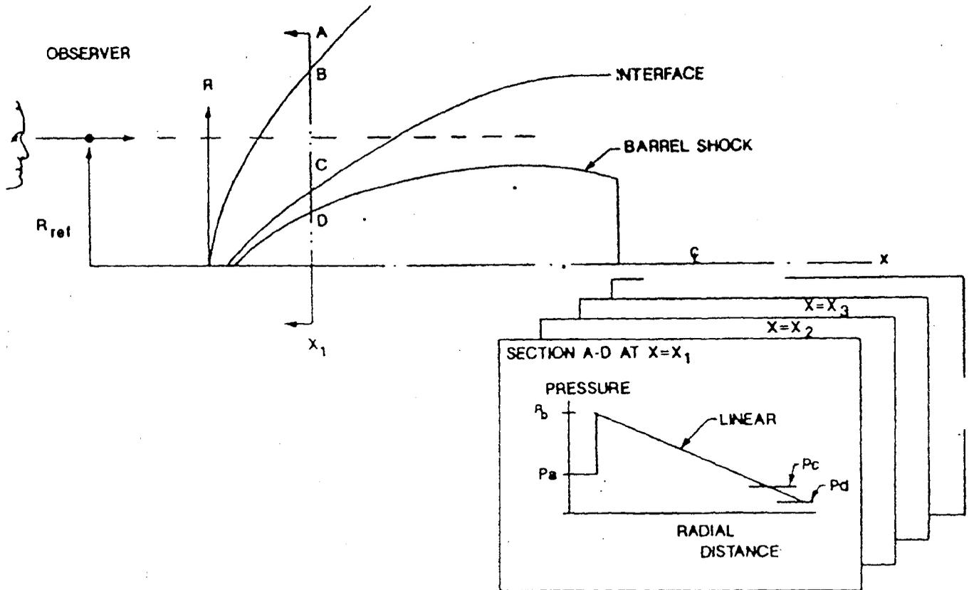
Figure 2-9. Methodology for Pressures in Field Between Boundaries
