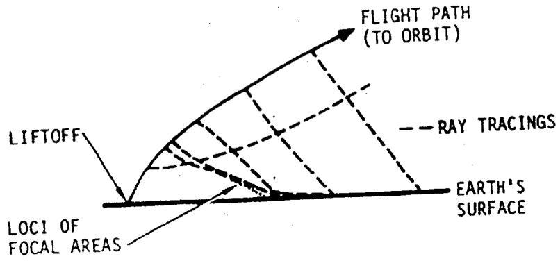
Figure 1-3. Shuttle Ascent Sonic Boom Propagation
