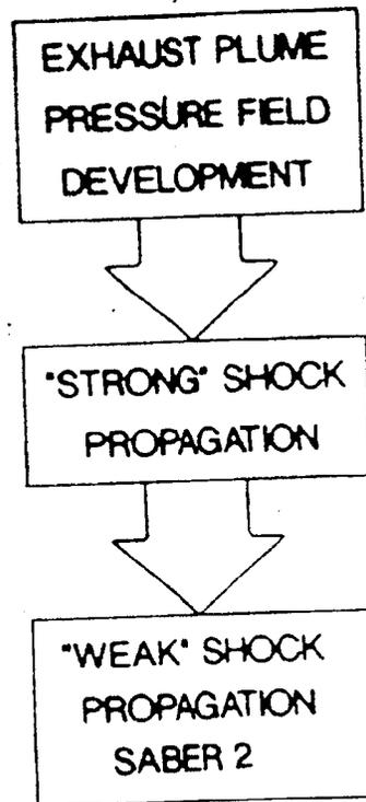
Figure 1-4. Primary Model Components
