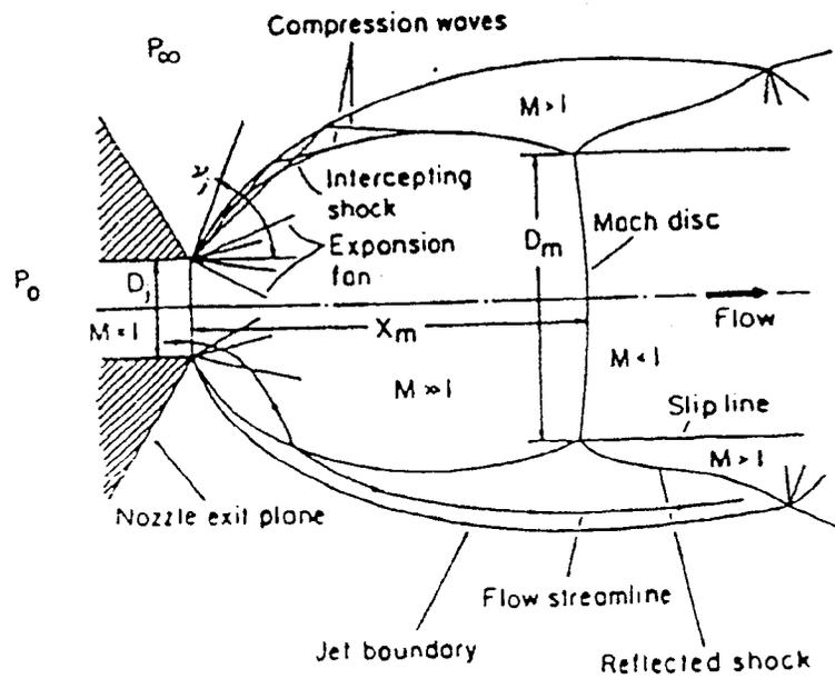
Figure 2-7. Schematic of Underexpanded Jet
