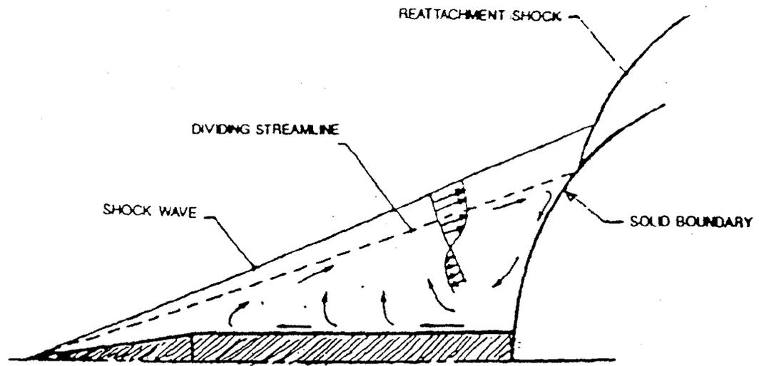
Figure 2-6. Comparison of Actual and Simulated Plume Induced Separation Region
