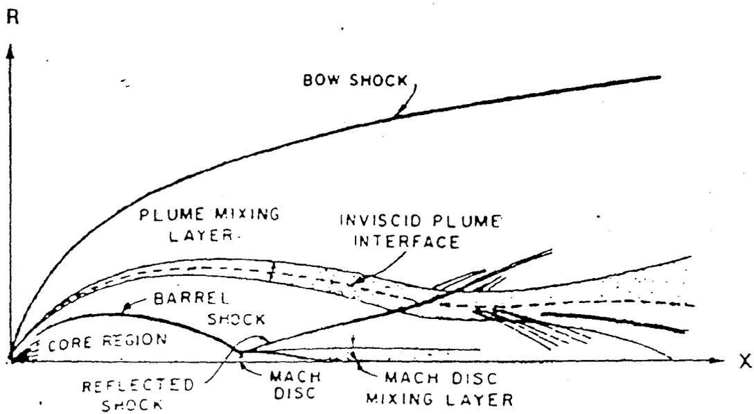
Figure 2-5. Schematic of Viscous/Inviscid Structure in Plume Nearfield
