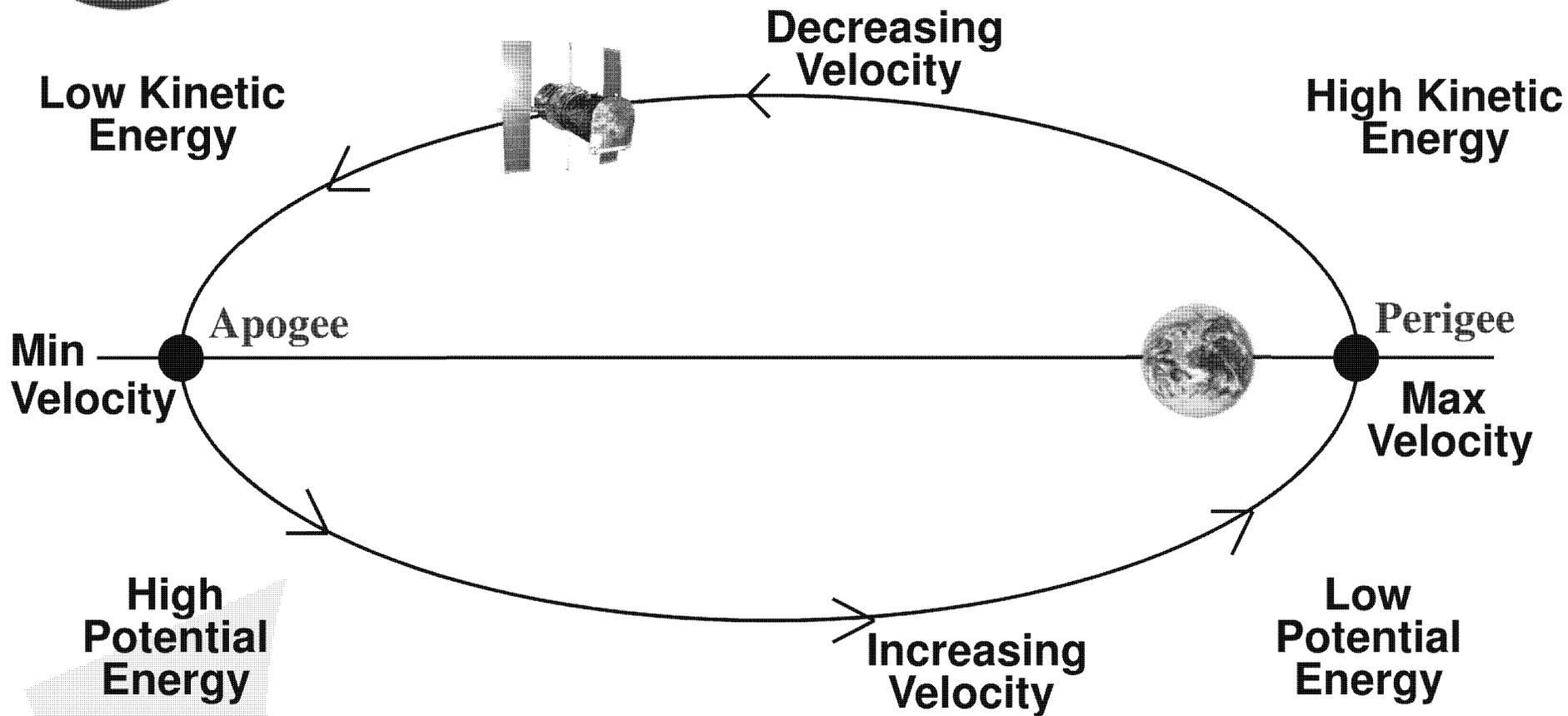
$$\text{Total Energy} = \text{Kinetic Energy} + \text{Potential Energy}$$
