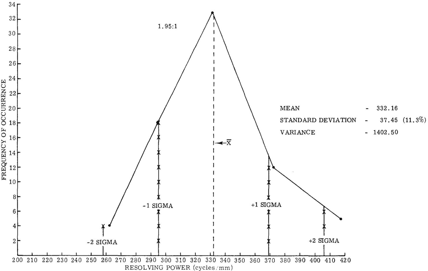
NOTE: This test was made on 3414 Film Type which was processed dual gamma in a Yardleigh Processor.
