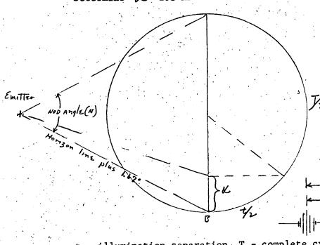
Assumption: Motion along circumference is constant, vertical component of motion defines the nod. Further assume, horizon line plus 1.67 degrees is base of circle (B).
