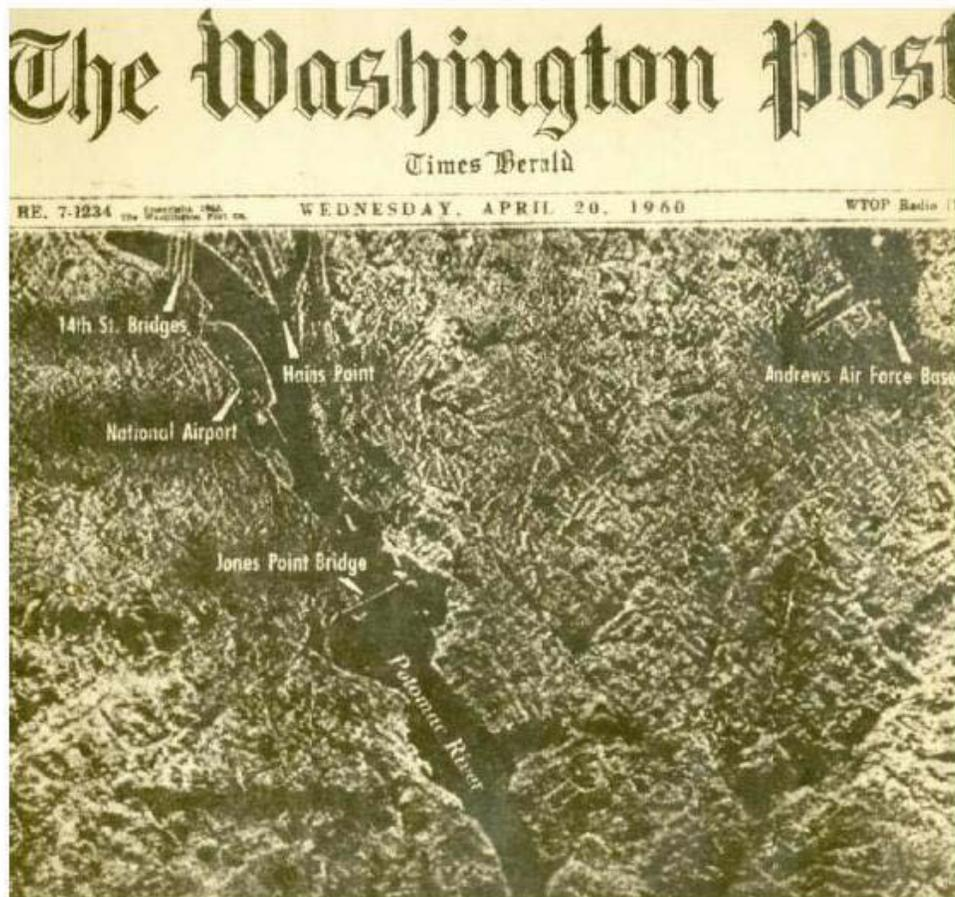
By April of 1960 the potential for Synthetic Aperture Radar or SAR as an intelligence tool was displayed to the public. This is the front page of the Washington Post, it shows an image taken by an aircraft mounted ANUPD-1 Side Looking Radar of Washington D.C.
