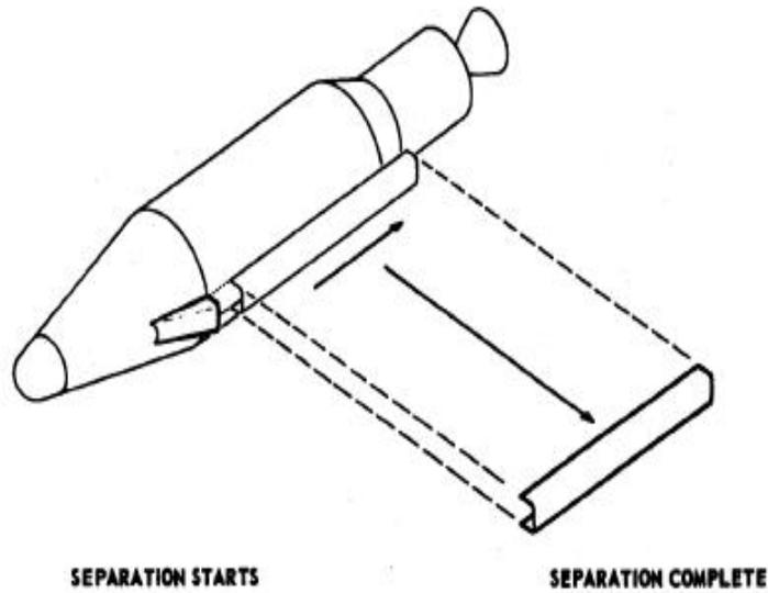
Figure 2.1.1.6 Vehicle Fairing Separation
