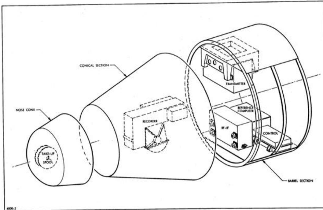
Figure 14 - KP-II Side-Looking Radar Installed in Forward Section of Agena Vehicle
