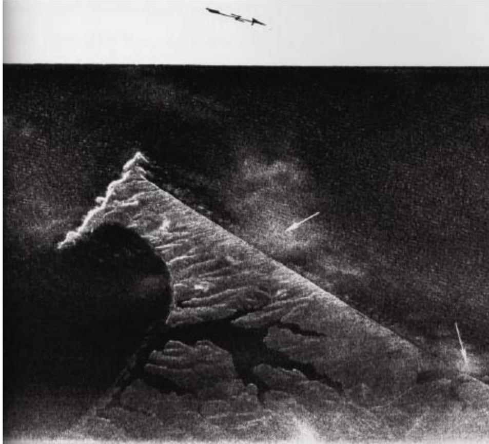
The arrows here indicate dense rain squalls, visibility in those rain squalls was under  $\frac{1}{4}$  of a mile. But you can still discern dominant wave patterns; you can see the surf lines off Point Reyes. You can see how the surf curves around the Point. This is just an experiment, the potential here is truly remarkable for 1964. No imagery satellite could have penetrated that cloud cover.  $\frac{1}{4}$  mile of visibility in the storms and you can still discern useful information.
