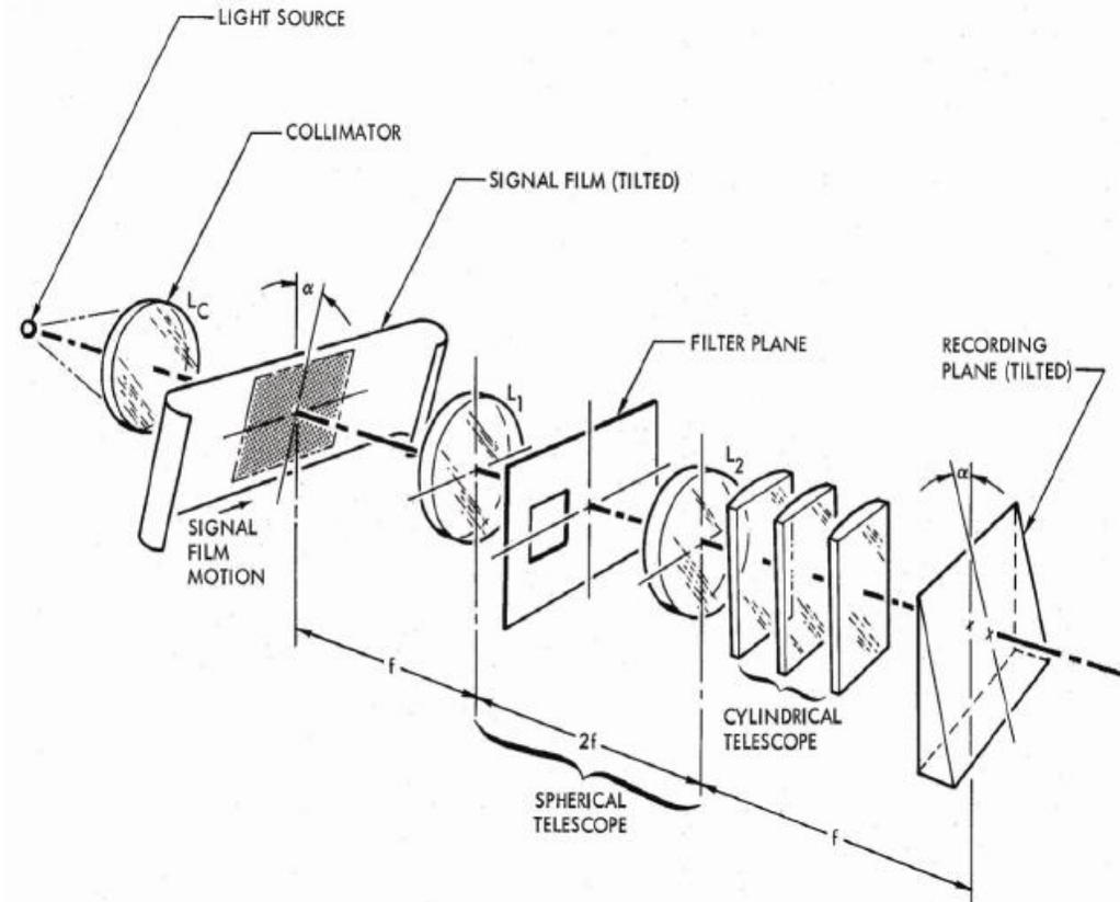
And that's what the Precision Optical Processor, the POP, actually does inside it: Simply an array of lenses, prisms, a focal plane and lasers for illumination sources. By running the transparency through this, you can expose another set of film, get a duplicate and analyze it.
