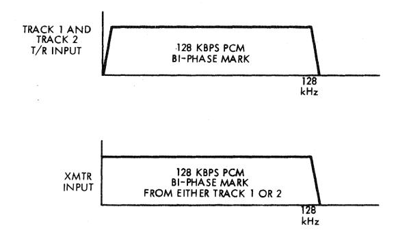
Fig. 3-3 Data Format: 1:1 Readout Mode (Narrowband PM Mode)
