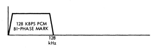
Fig. 3-4 Transmitter Input: Realtime Transpond Mode
