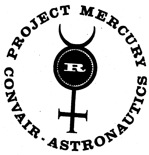
Figure 4. (above) Design used to identify components which have been subjected to "added reliability" selection and inspection requirements for Project MERCURY. Symbol in center is astronomical representation used for mercury. R in circle is a "reliability reminder."
