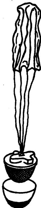
PARACHUTE DEPLOYMENT—ABLATION SHIELD SEPARATION
