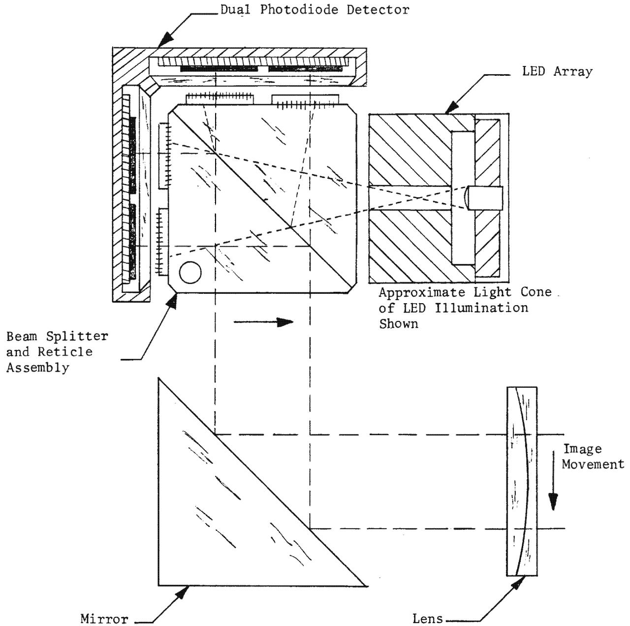
Figure 3.6-11. Optics with Dual Detector and LED Array
