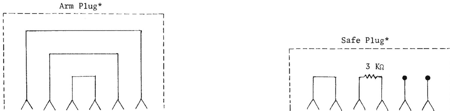
\*Simplified schematic showing one pyro and the continuity loop.
