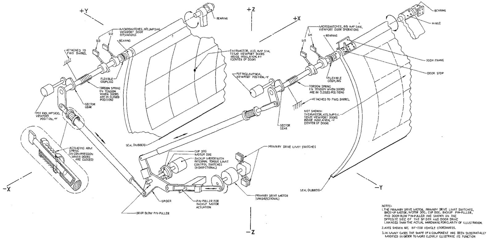
Figure 3.5-3. Viewport Door Drive Mechanism and Instrumentation
