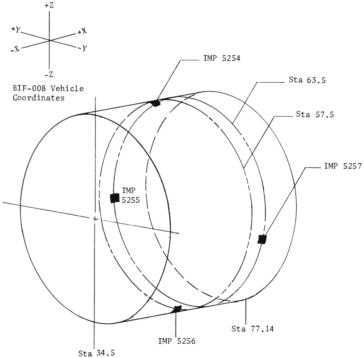
Figure 3.8-16. Supply Electronics Module Skin Temperature Instrumentation Points
