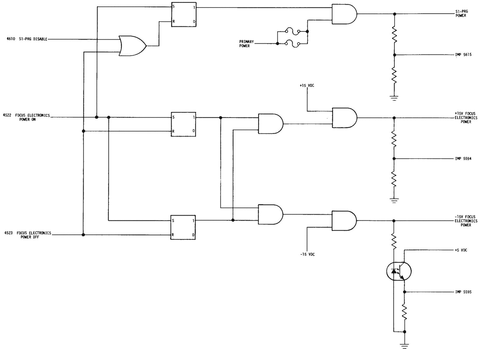
Figure 3.7-8. Focus Electronics and S1-PRG Power
