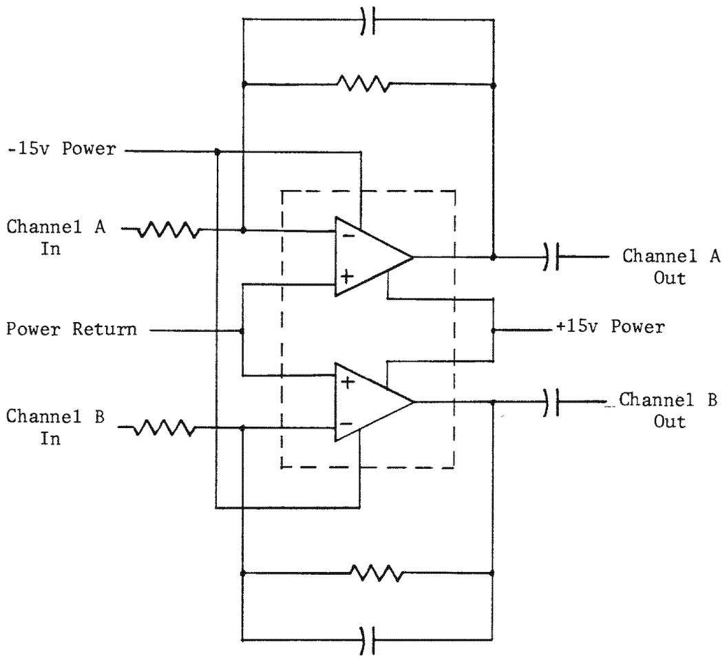
Figure 3.6-15. Typical Dual Channel Amplifier
