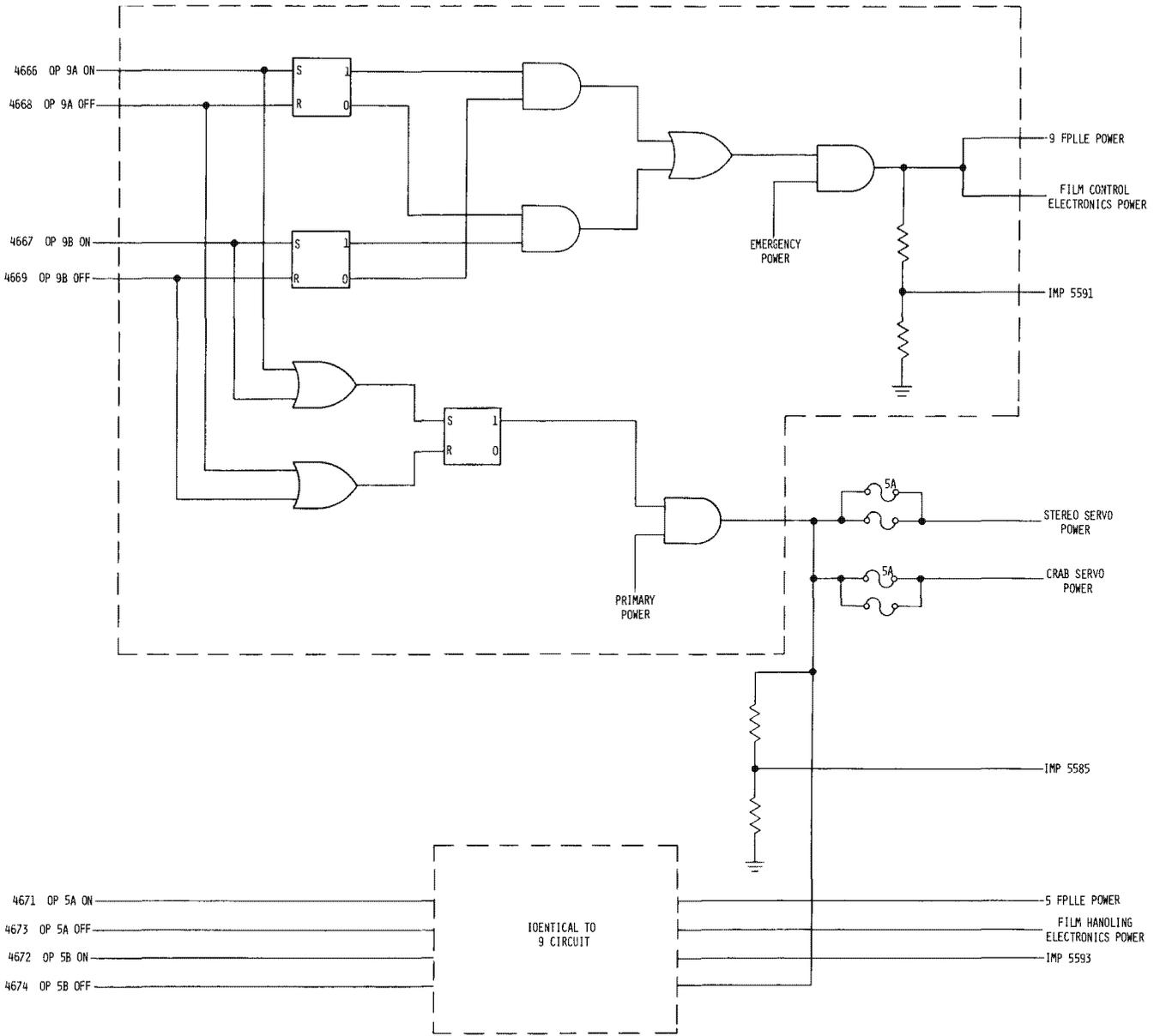
Figure 3.7-7. 9 and 5 Operational Power and Servo Power
