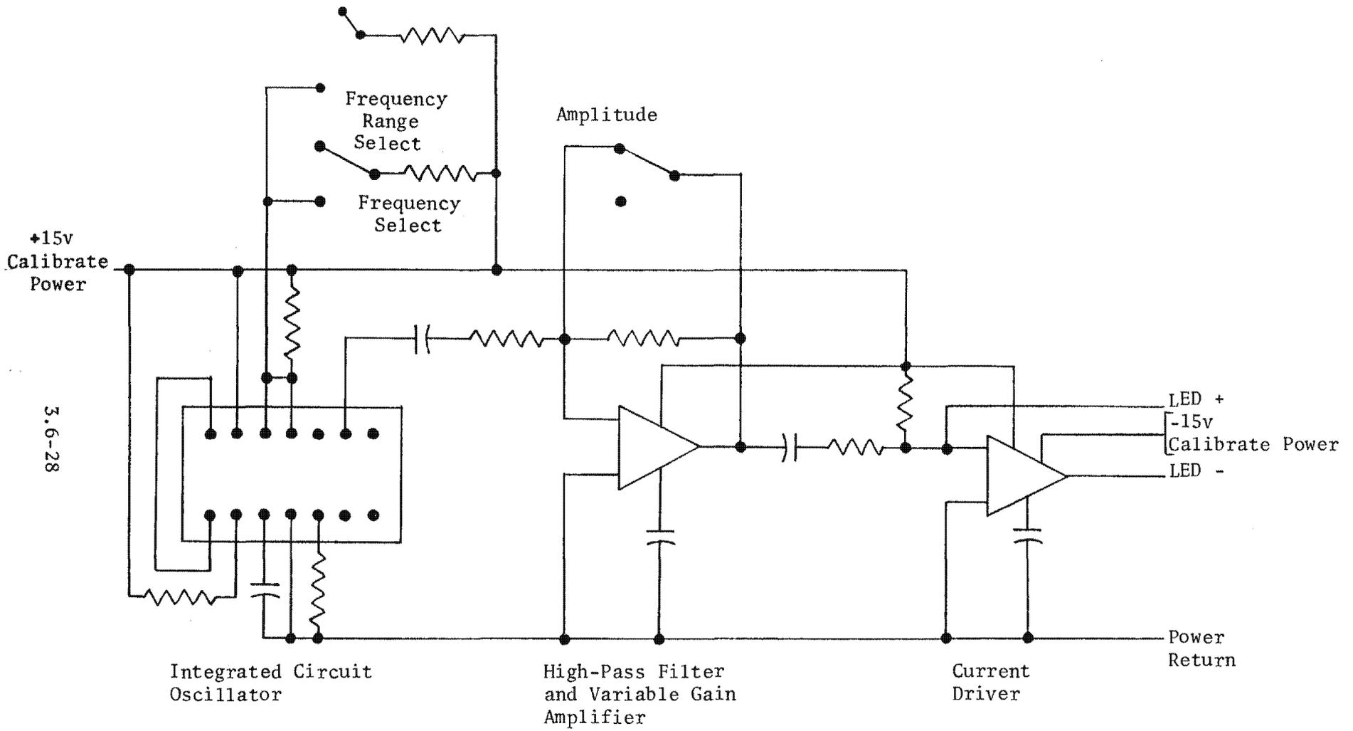
Figure 3.6-18. LED Oscillator and Driver
