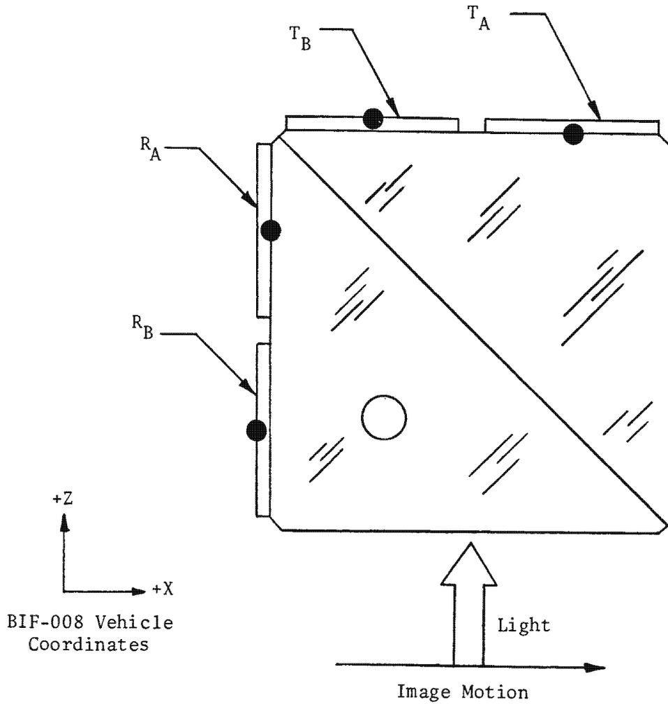
Figure 3.6-6. Beam Splitter and Reticule Assembly
