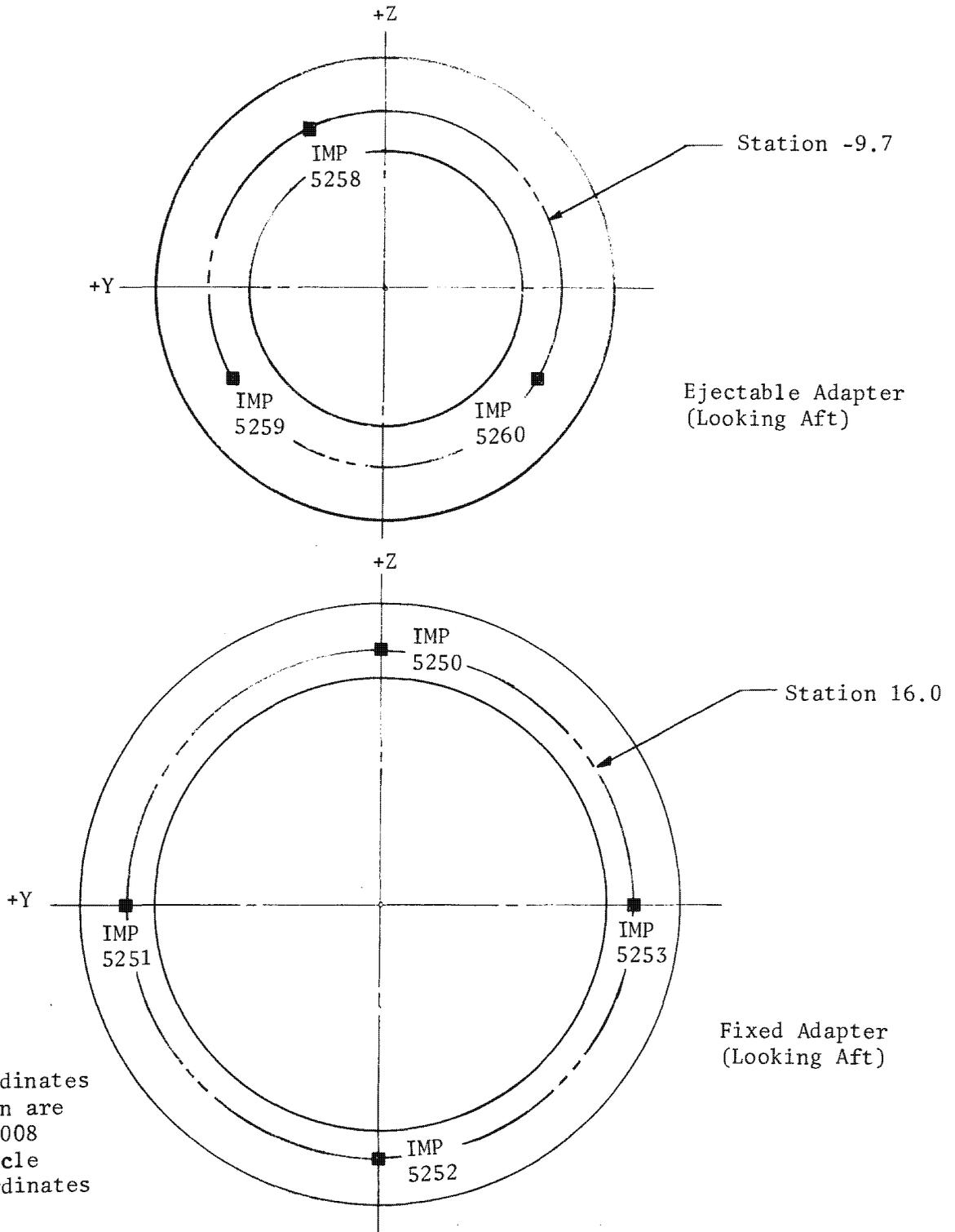
Figure 3.8-15. DRM Skin Temperature Instrumentation Points
