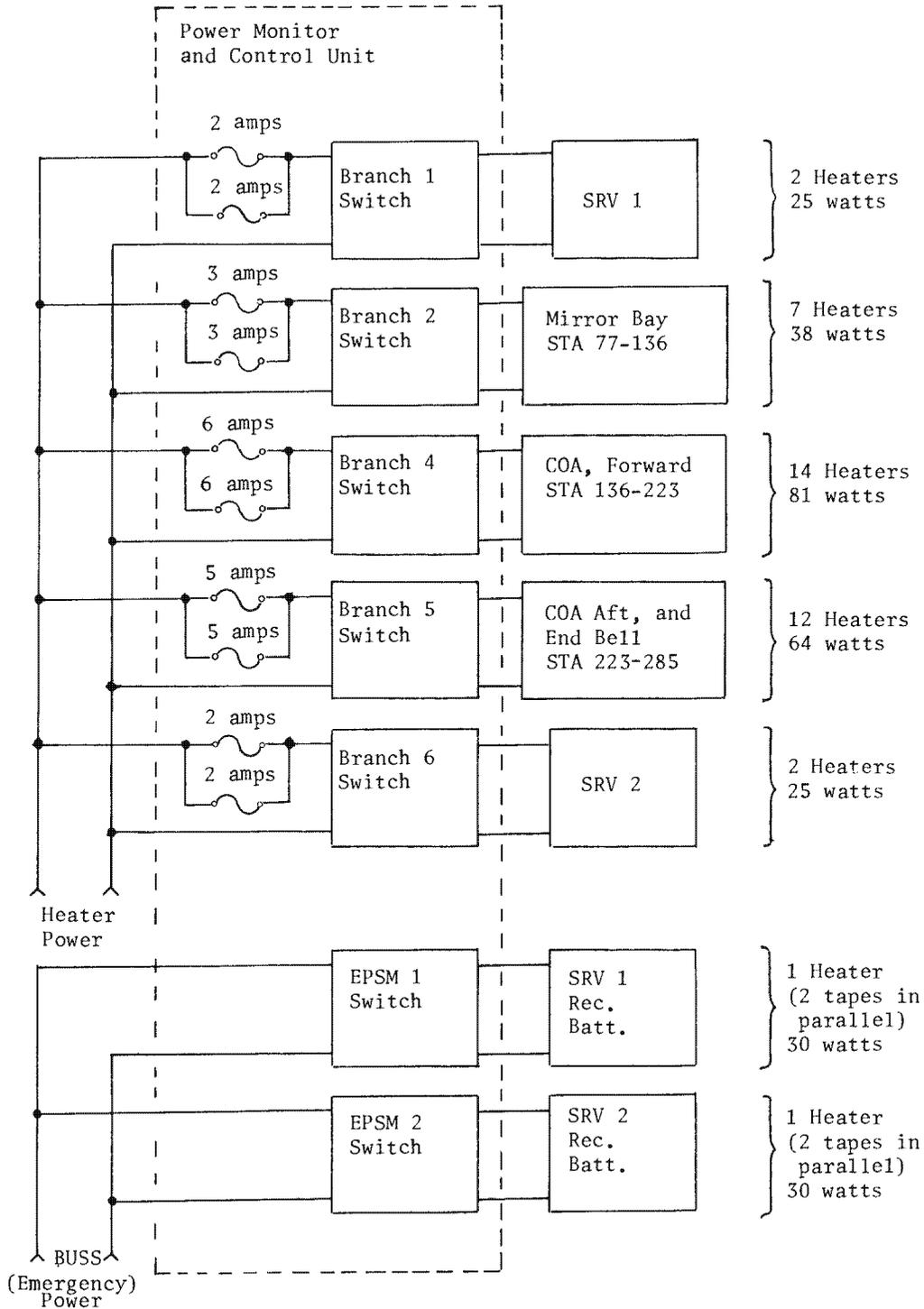
Figure 3.8-10. Flight Heater Branch Block Diagram
