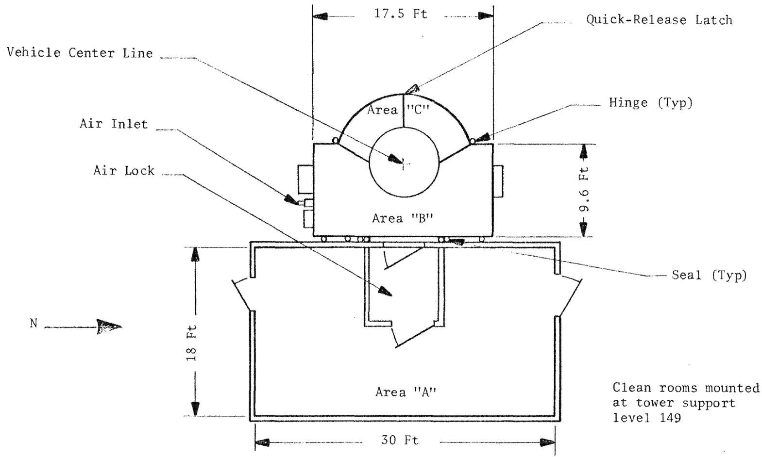
Figure 3.8-3. Floor Plan, Gantry Clean Rooms
