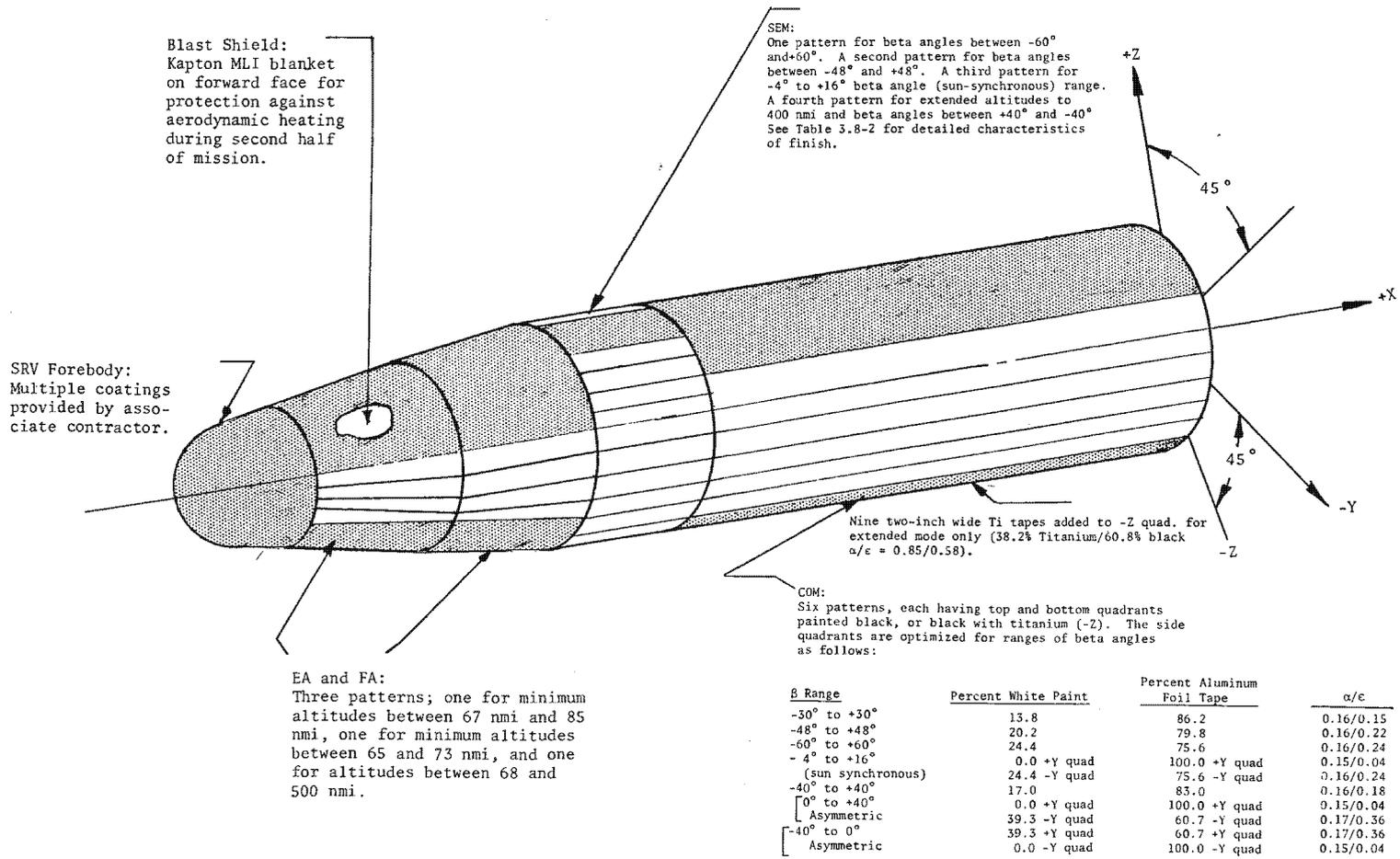
Figure 3.8-6. PPS/DP EAC External Thermal Control Finishes
