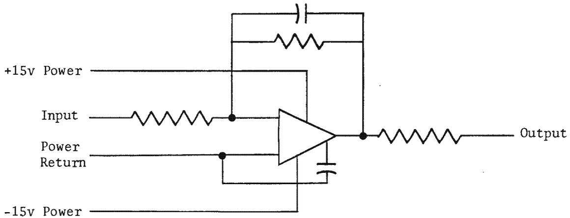
Figure 3.6-17. Typical Scaling Amplifier and Low-Pass Filter
