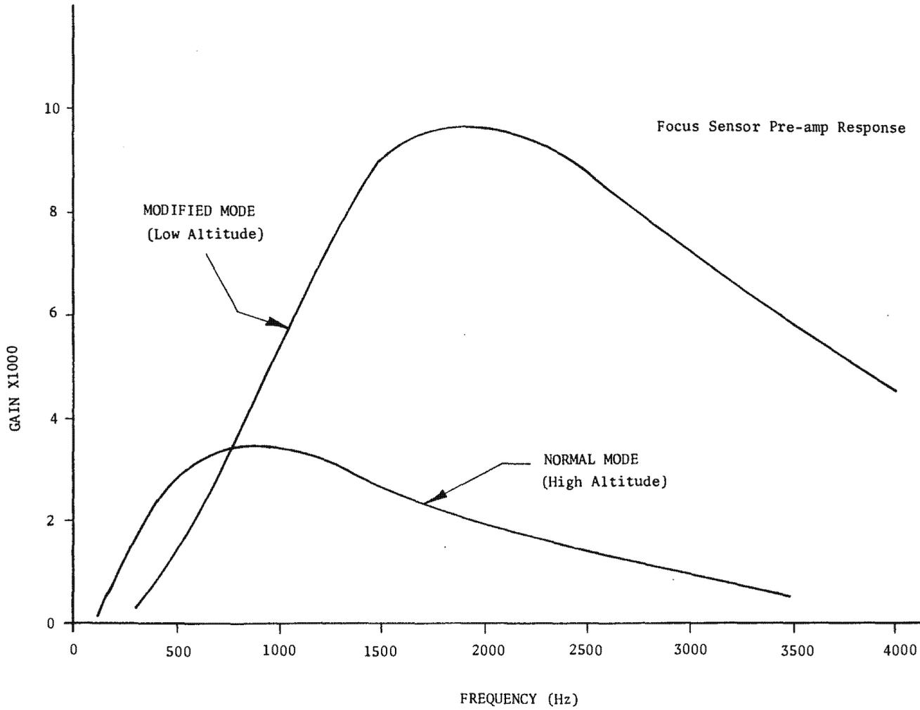
Figure 3.6-14. Frequency Response for Each Mode
