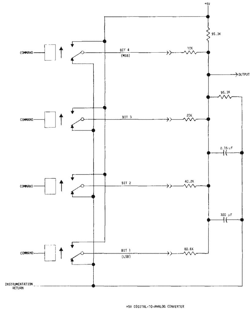
Figure 3.7-21. Command Receipt Instrumentation Digital-to-Analog Converters
