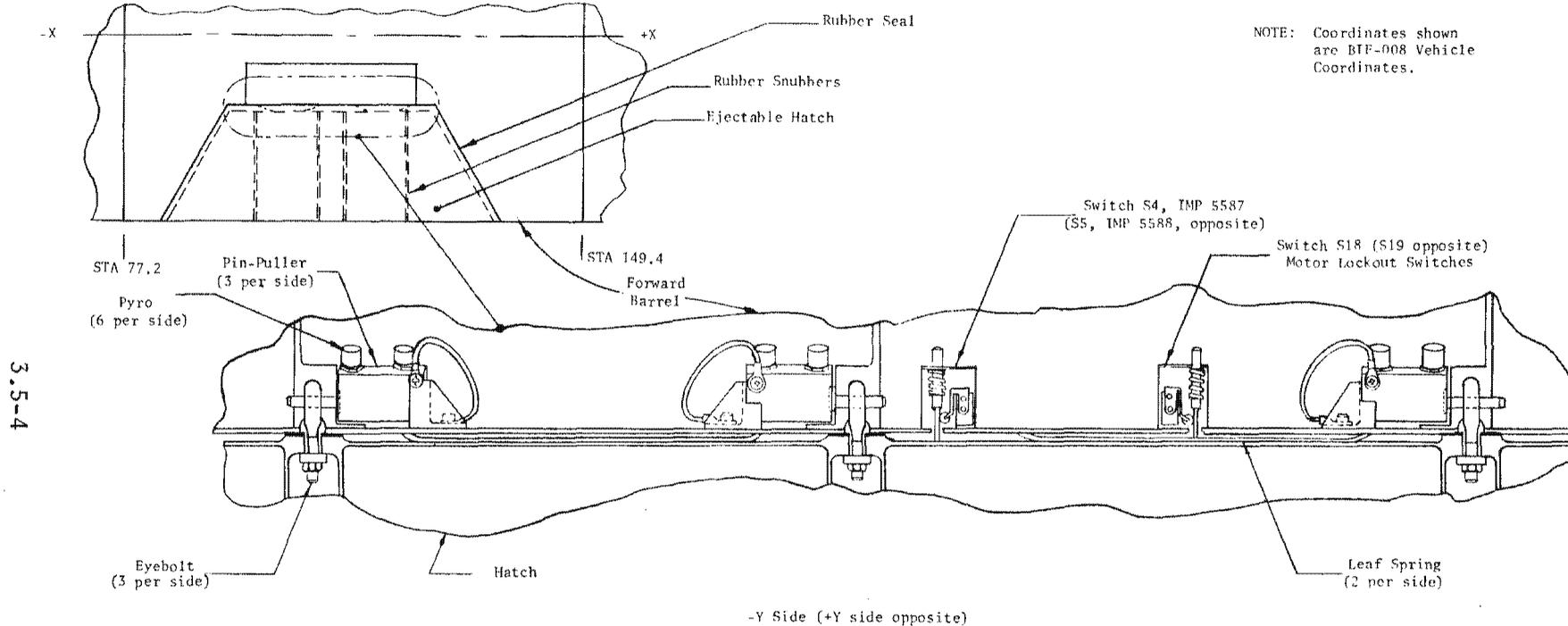
Figure 3.5-2. Hatch Ejection Mechanism
