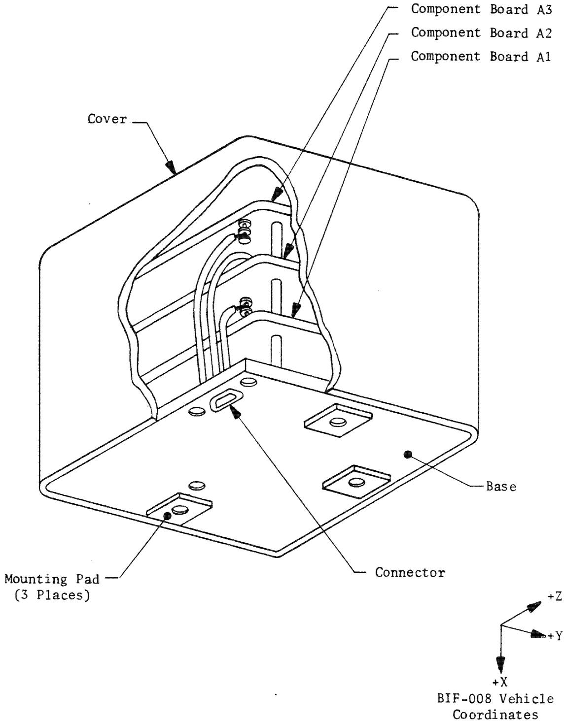
Figure 3.6-8. Signal Normalizing Module (Unit 15A3)
