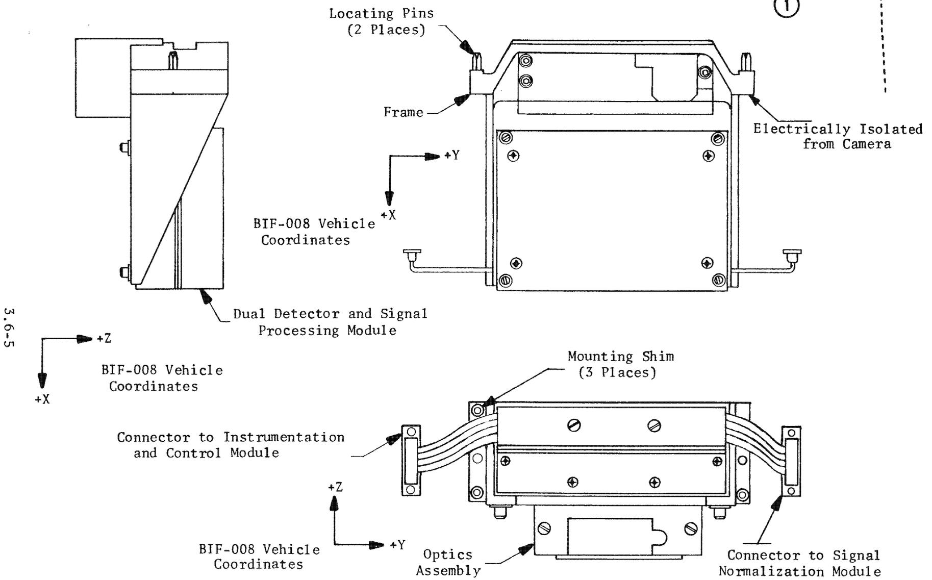
Figure 3.6-4. Focus Sensor Head Assembly
