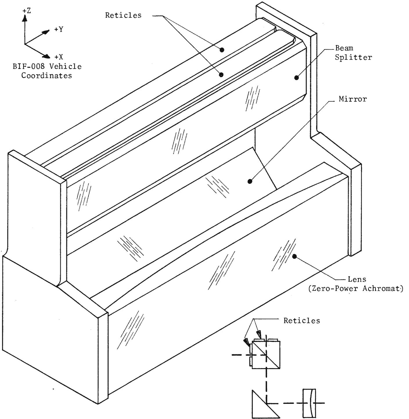
Figure 3.6-5. Focus Detection Subsystem Optics Assembly
