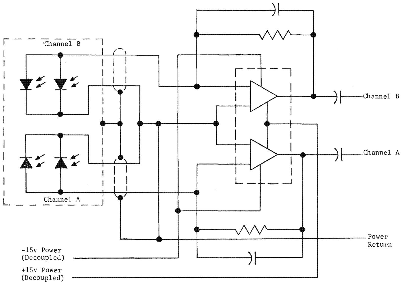
Figure 3.6-13. Detector and Current-to-Voltage Converter
