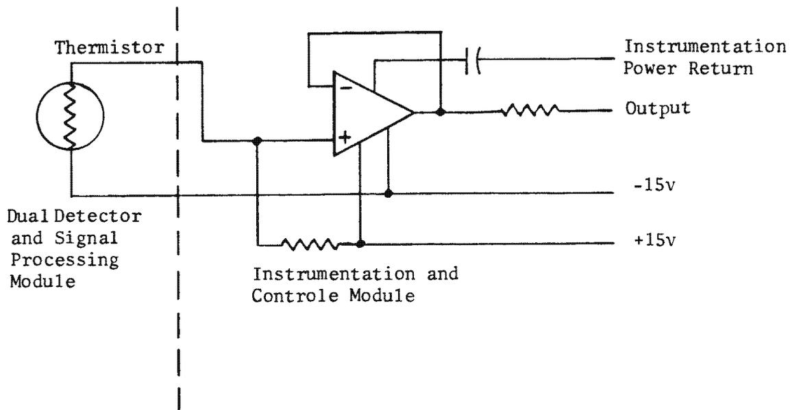
Figure 3.6-19. Temperature Sensor Bias Network
