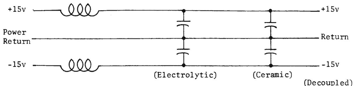
Figure 3.6-20. Power Decoupling Circuit
