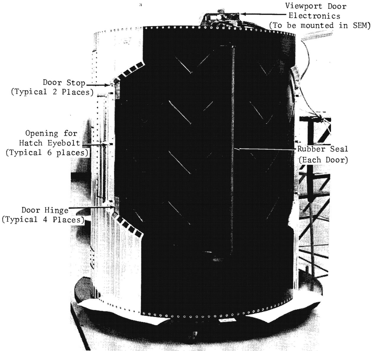
NOTE: Figure 3.1-20 in Part 3, Section 1 illustrates the forward barrel with the viewport doors open.
