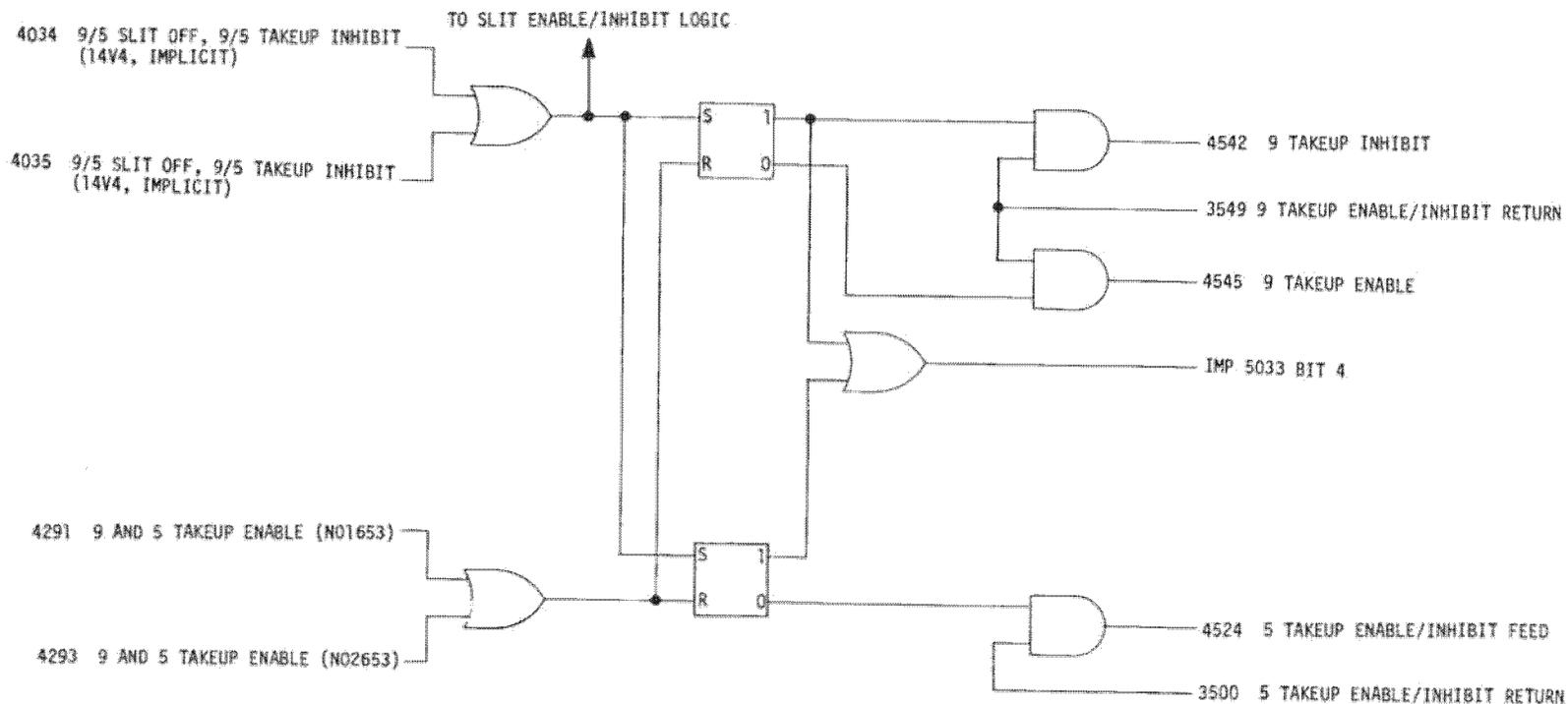
Figure 3.9-38. 9/5 Takeup Enable/Inhibit
