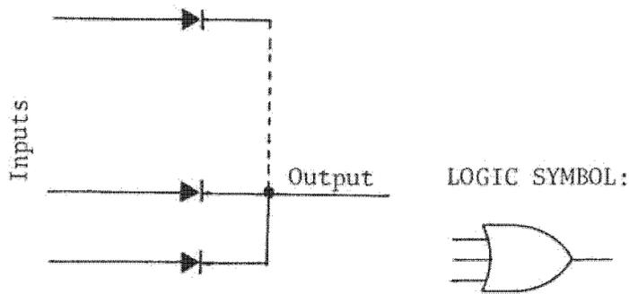
Figure 3.9-15. Command Input Diode OR Gate
