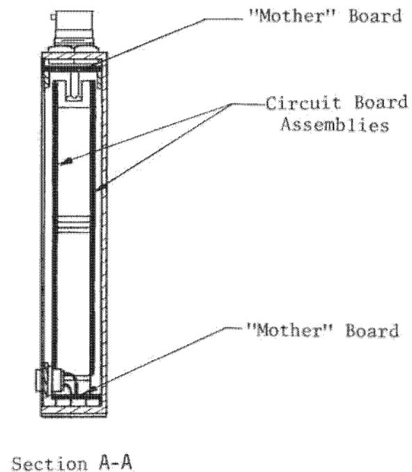
Figure 3.10-22. Converter Unit Mechanical Construction
