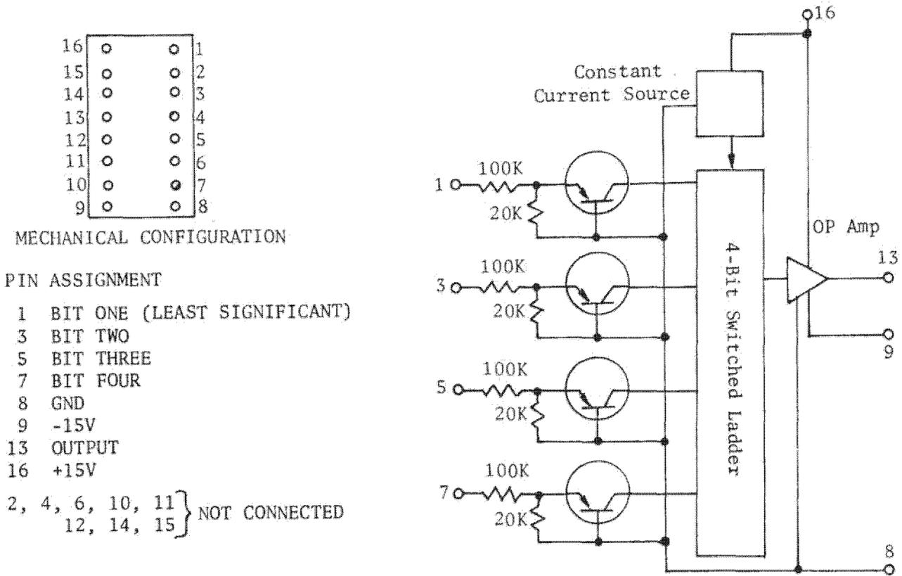
Figure 3.9-19. Instrumentation Digital-to-Analog Converter
