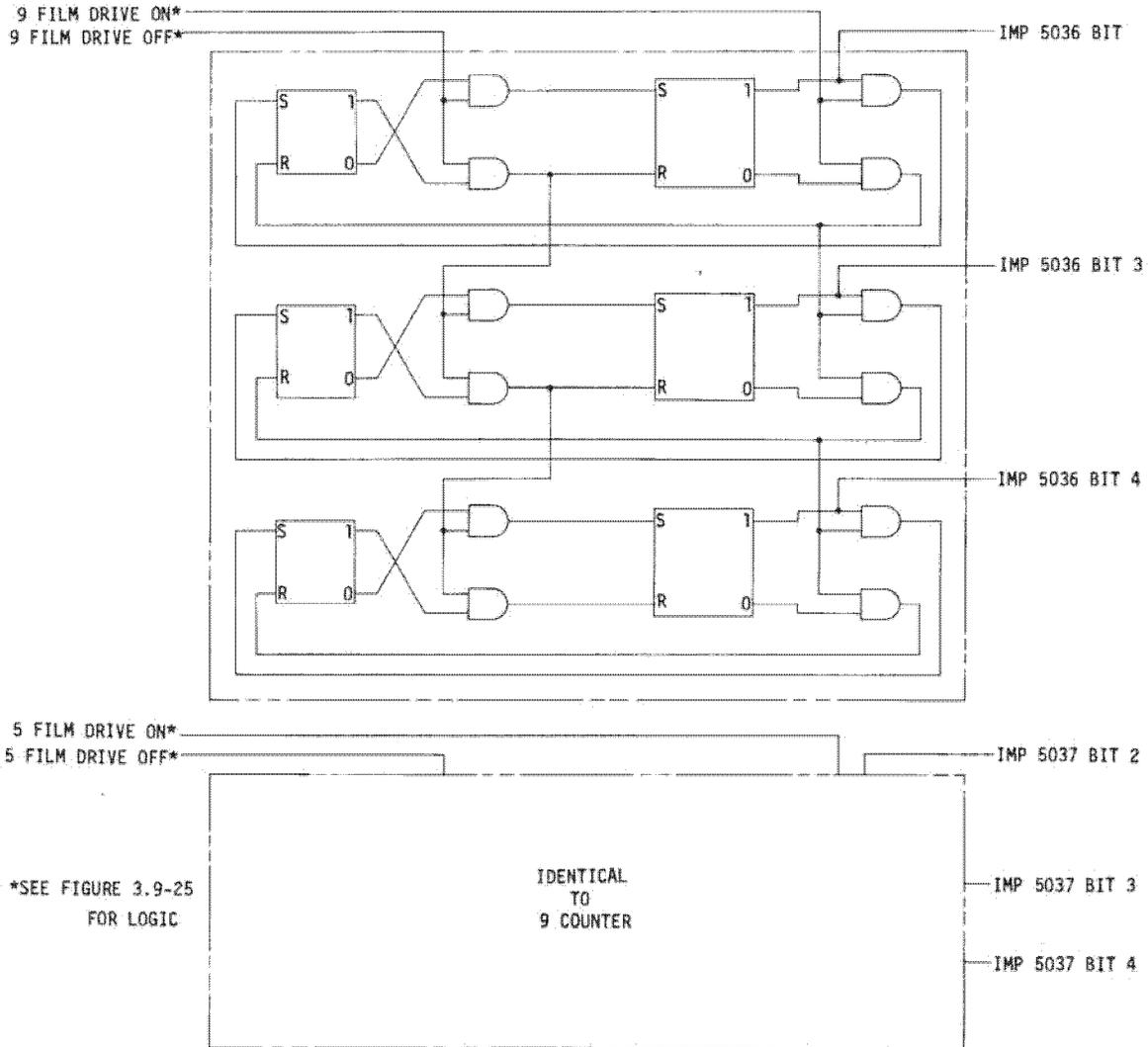
Figure 3.9-26. 9 and 5 Camera Operations Counters
