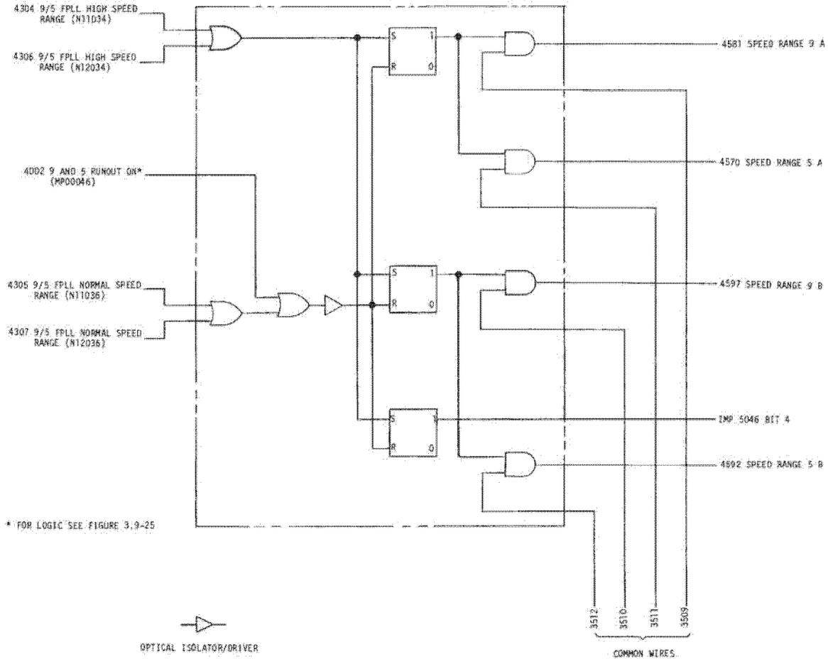
NOTE: See Figure 3.9-48 for a logic description of CP Commands which revise film-drive speeds for high altitude modes.
