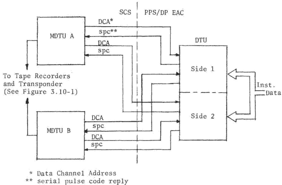
Figure 3.10-18. MDTU/DTU Interface
