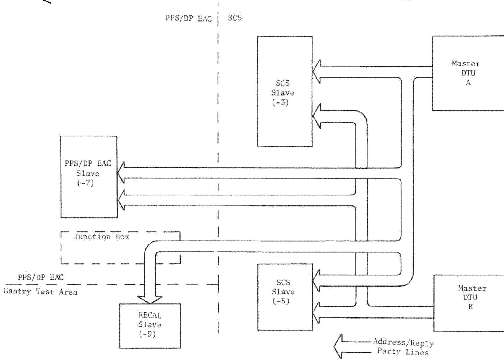
Figure 3.10-38. PSV Slave and Master Telemetry Units
