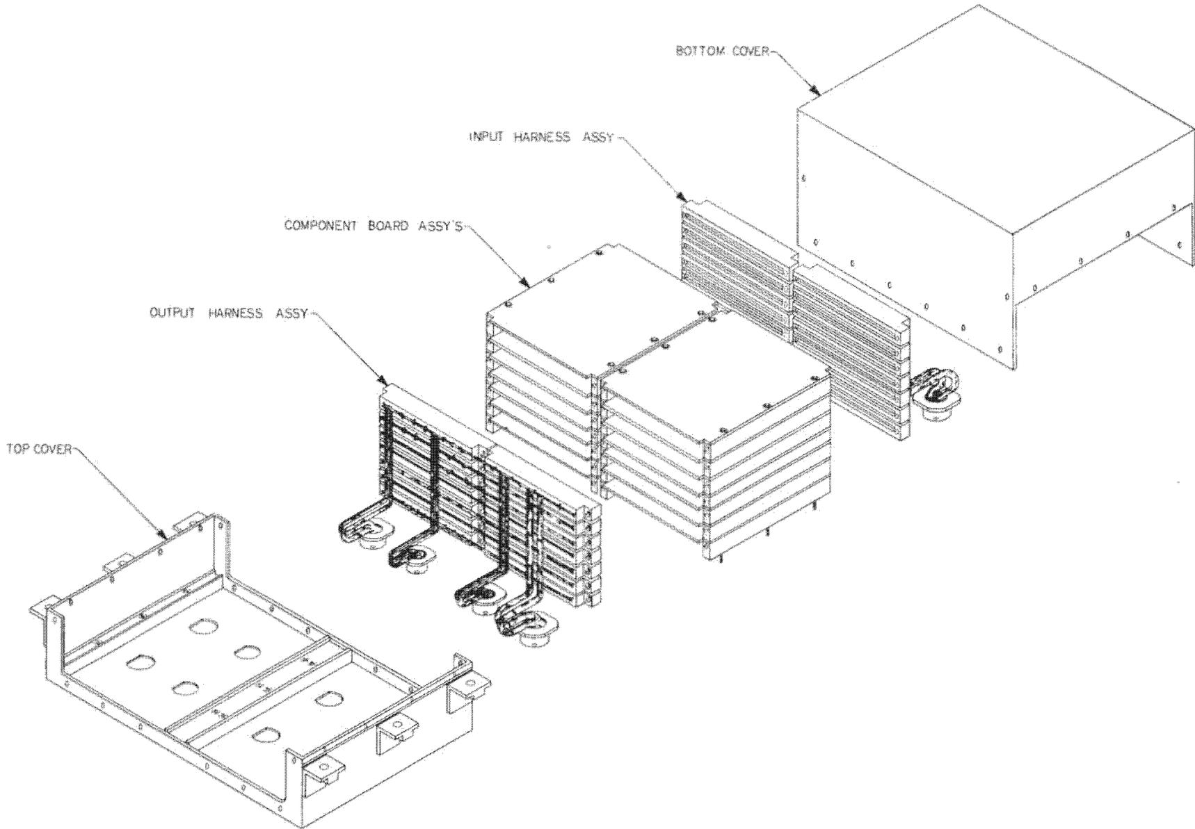
Figure 3.9-13. Command Processor Assembly
