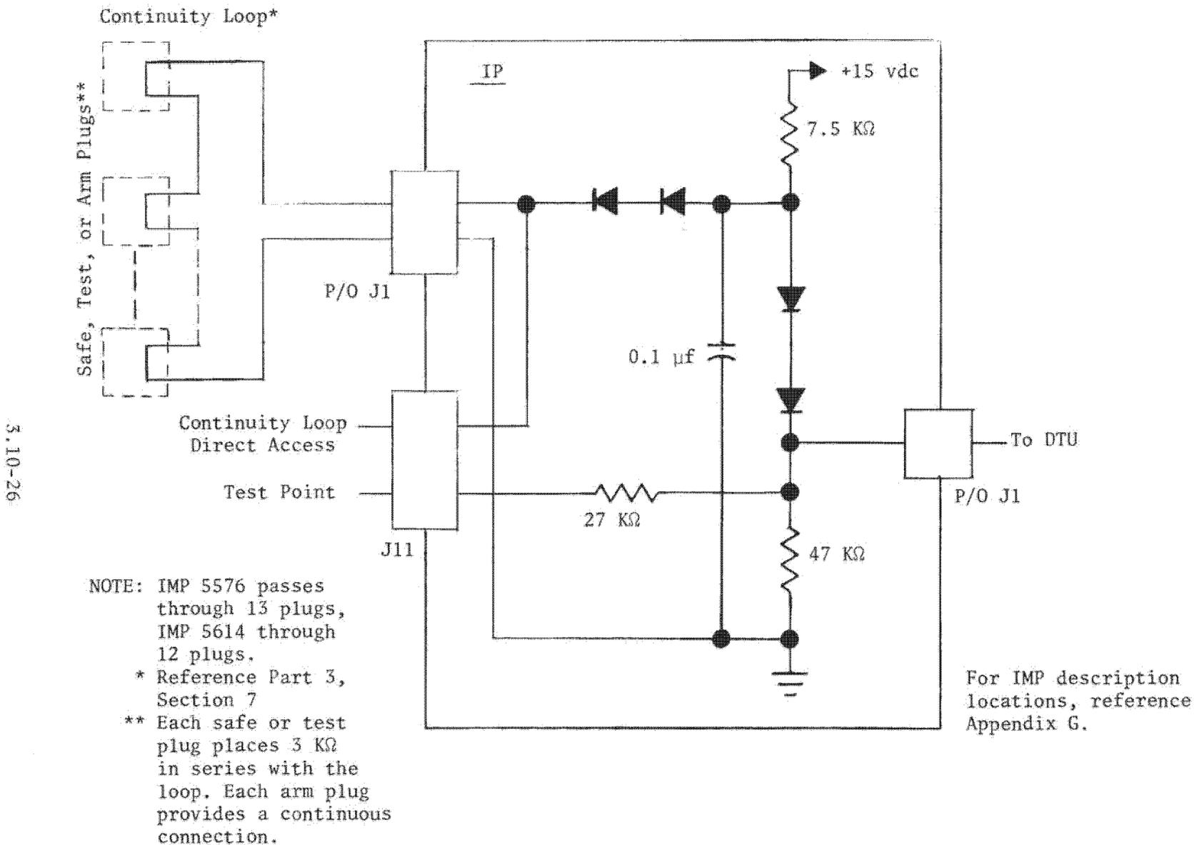
Figure 3.10-15. Typical IP Processing Circuit: IMP's 5576 and 5614
