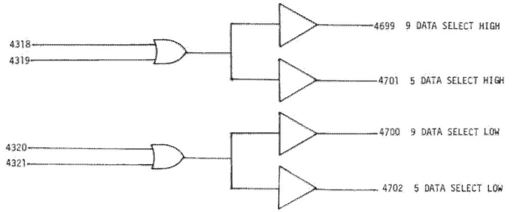
Figure 3.9-49. High/Low Altitude Select SRC Common and Data Lamp Select
