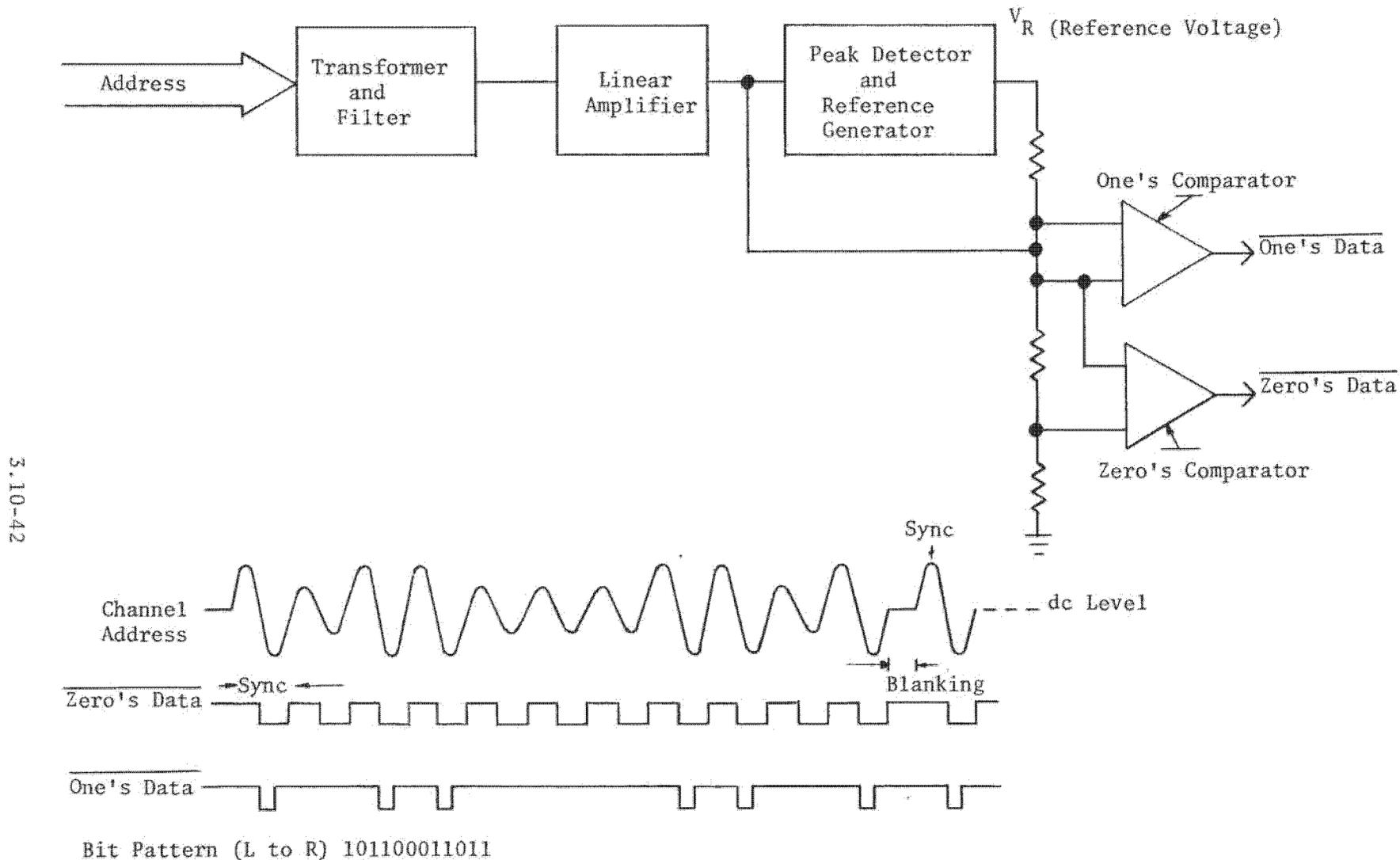
Figure 3.10-25. Address Receiver Block Diagram
