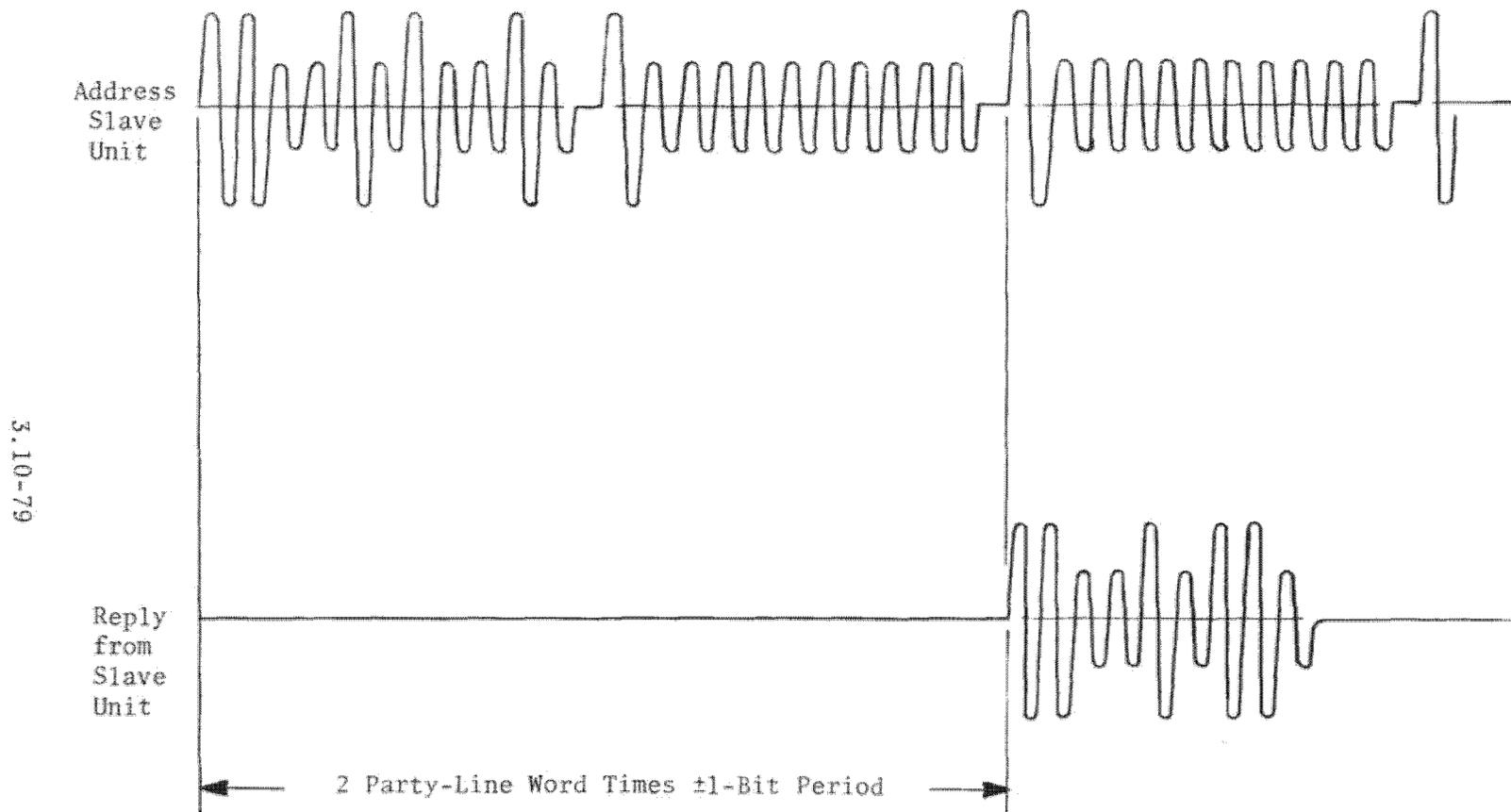
Figure 3.10-41. Time Relationship: Remote Channel Address Code/Serial Pulse Code Data Reply
