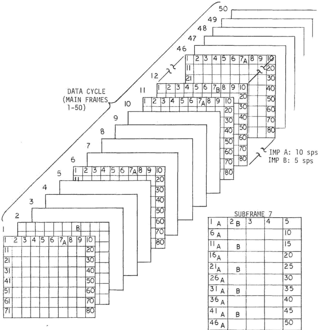
Figure 3.10-45. Format Example: 10 sps and 5 sps Monitors
