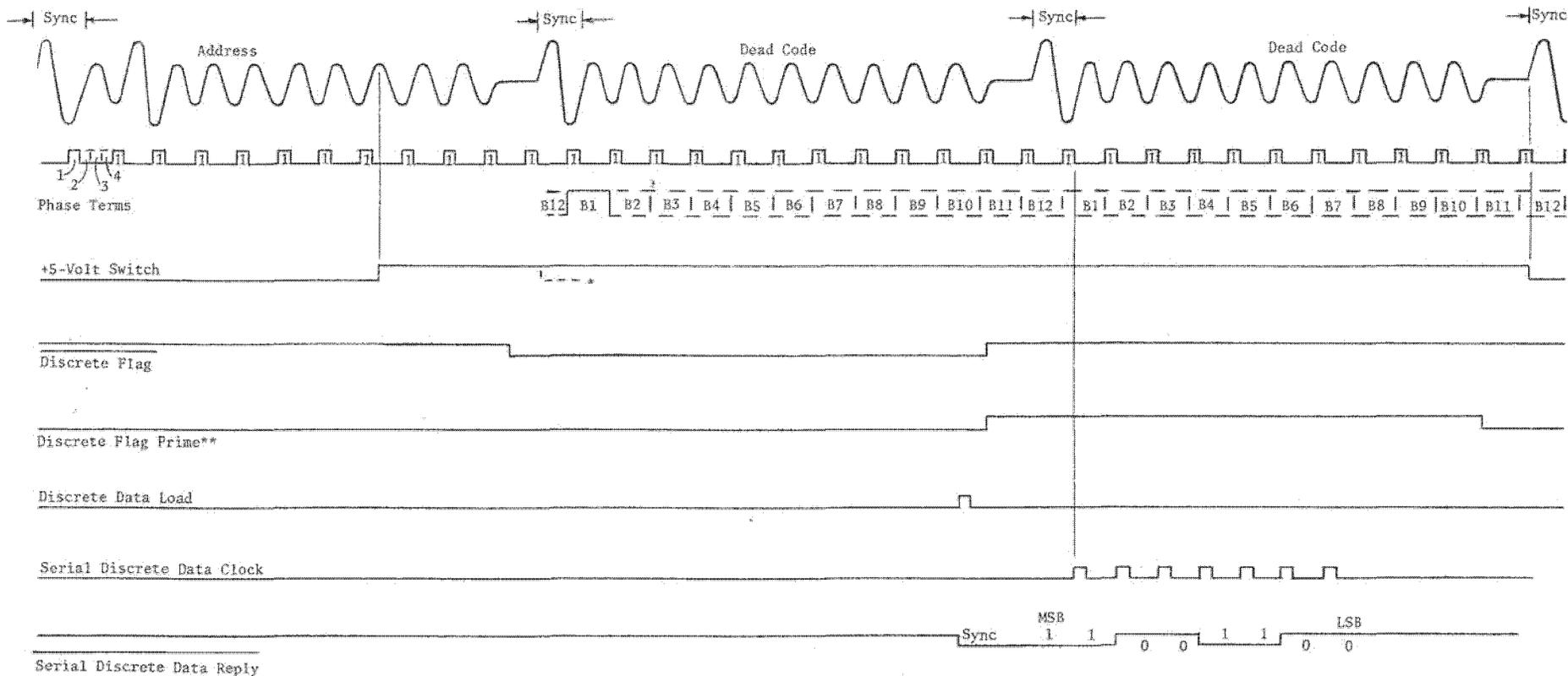
NOTE: Assumes at least three dead codes precede and follow the address (10-00<sub>g</sub>). This insures the converter coming up from an unpowered condition and shutting down after reply. (A reply code of 063<sub>g</sub> is shown.)
