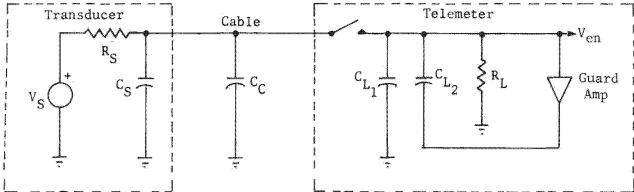
Figure 3.10-53. Sampling Transient Error Source
