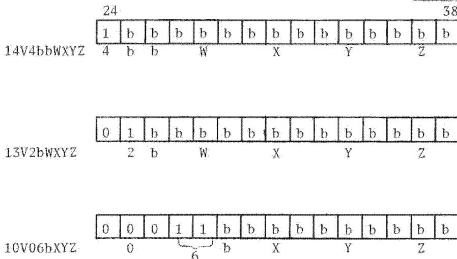
Figure 3.9-7. ECS 14V, 13V, and 10V VSPC Octal Codes
