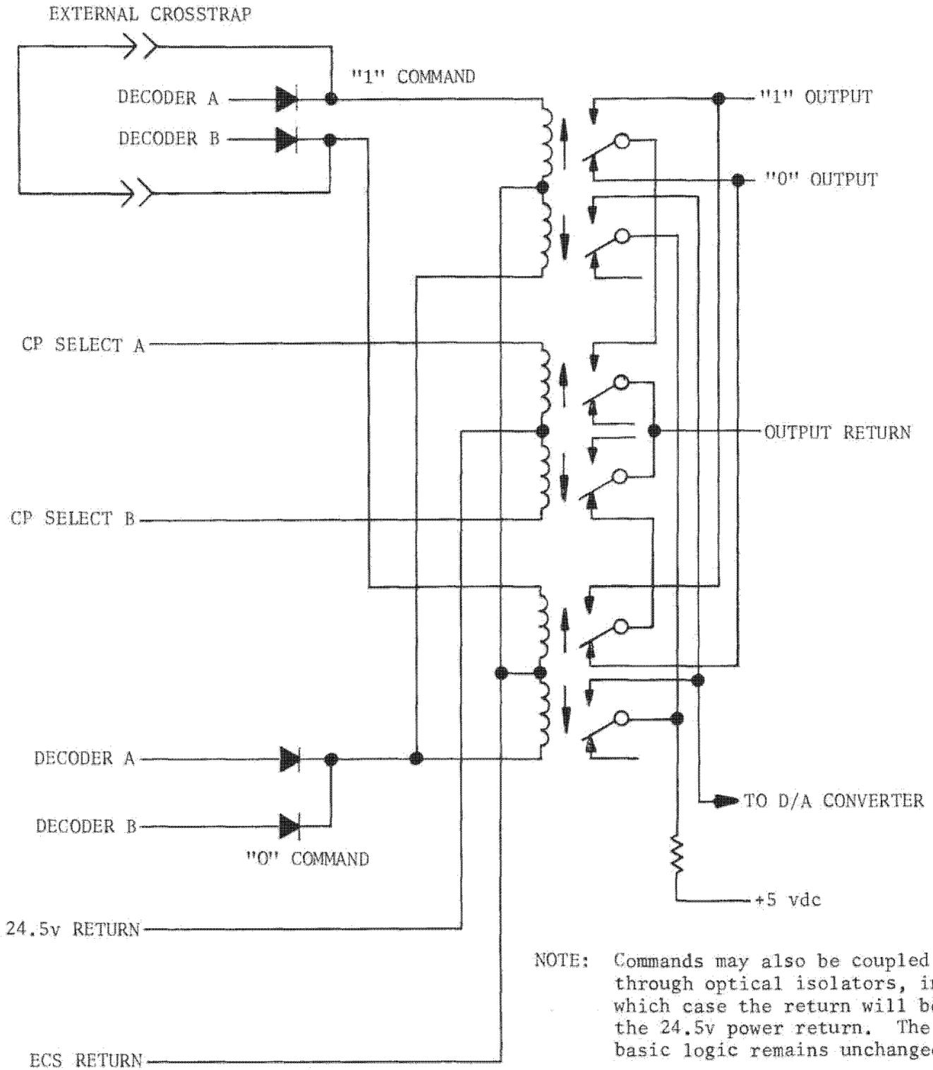
Figure 3.9-22. Basic Servo Mode Switch Circuit
