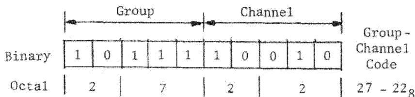
Figure 3.10-32. Group-Channel Address Code
