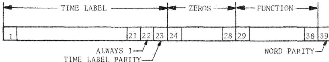
Figure 3.9-4. MCS Command Bit Structure
