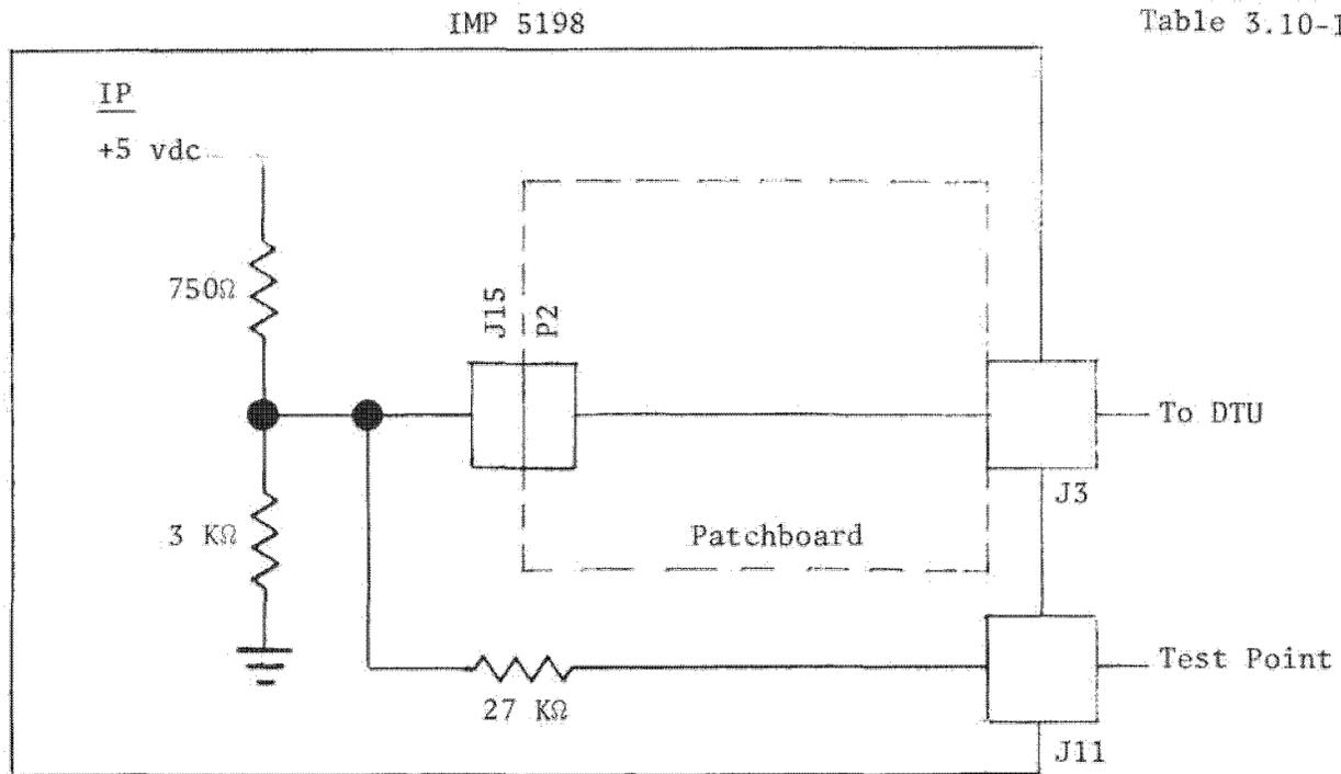
Figure 3.10-12. Generating Circuit: IMP's 5198 and 5200
