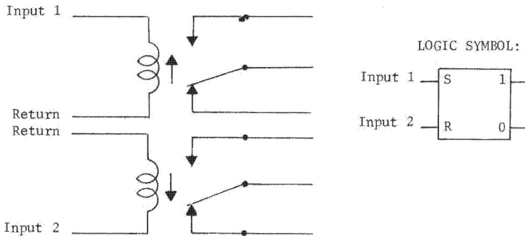
Figure 3.9-16. Latching Relay Logic Representation
