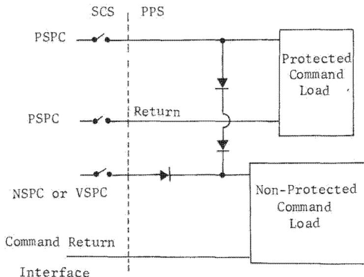
Figure 3.9-14. OR Gating Protected Commands with Non-Protected Commands
