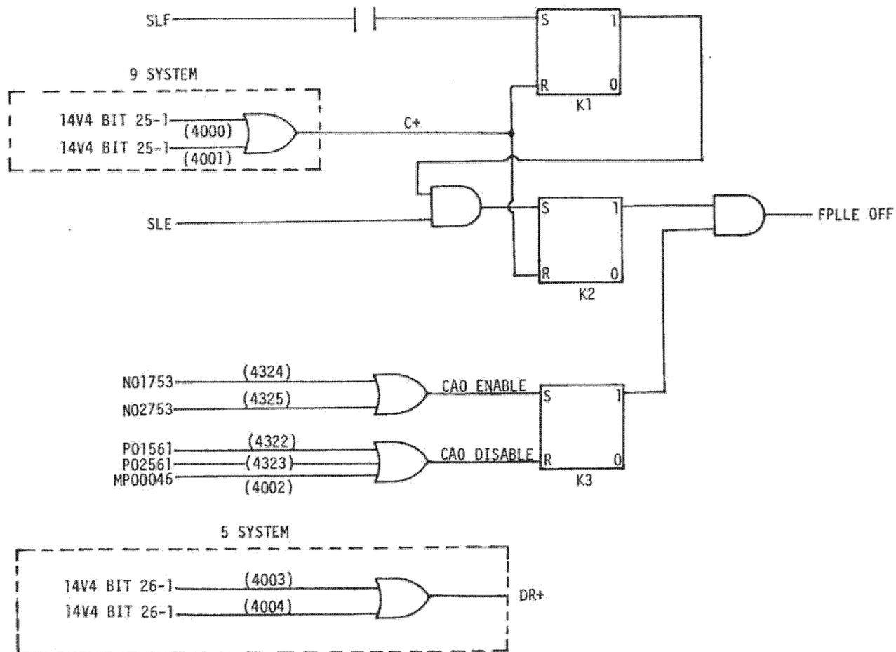
Figure 3.9-50. Camera Automatic Off Logic Diagram
