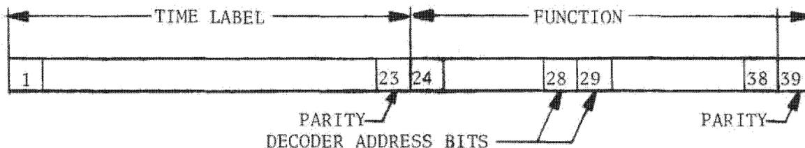
Figure 3.9-3. ECS Command Bit Structure
