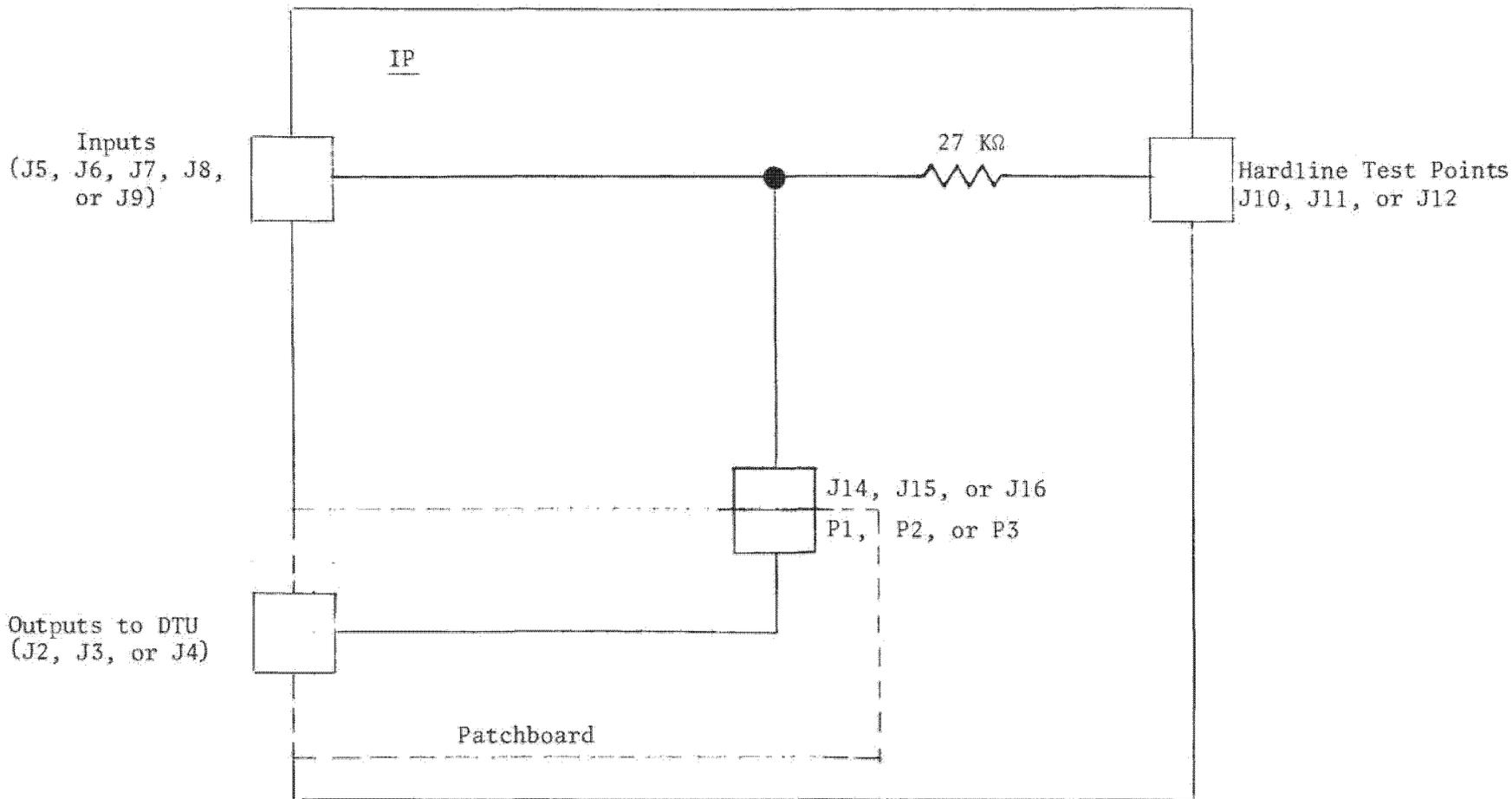
Figure 3.10-5. Typical Preprocessed Analog Signal IP Circuit
