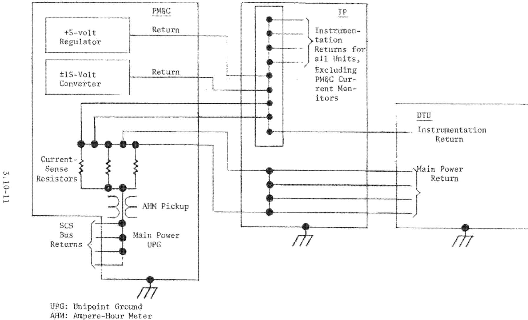
Figure 3.10-4. Instrumentation Unipoint Ground
