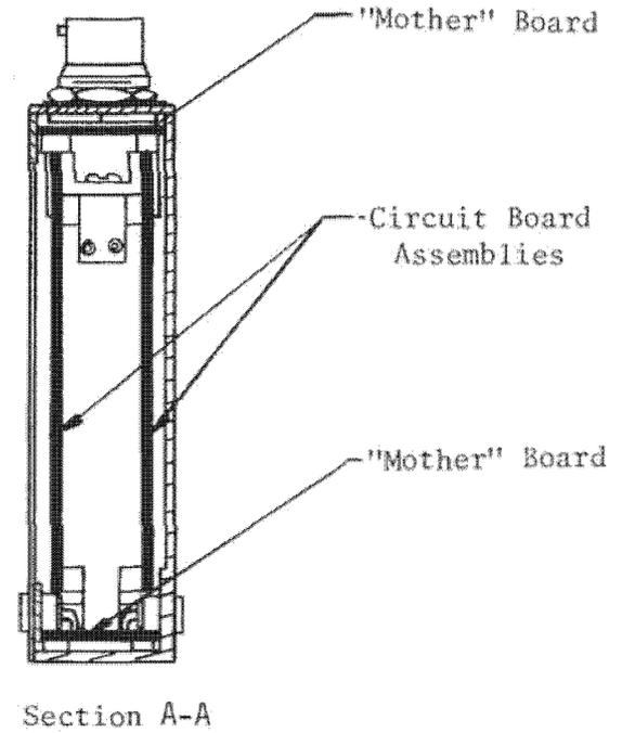
Figure 3.10-21. Typical AMU and DMU Mechanical Construction
