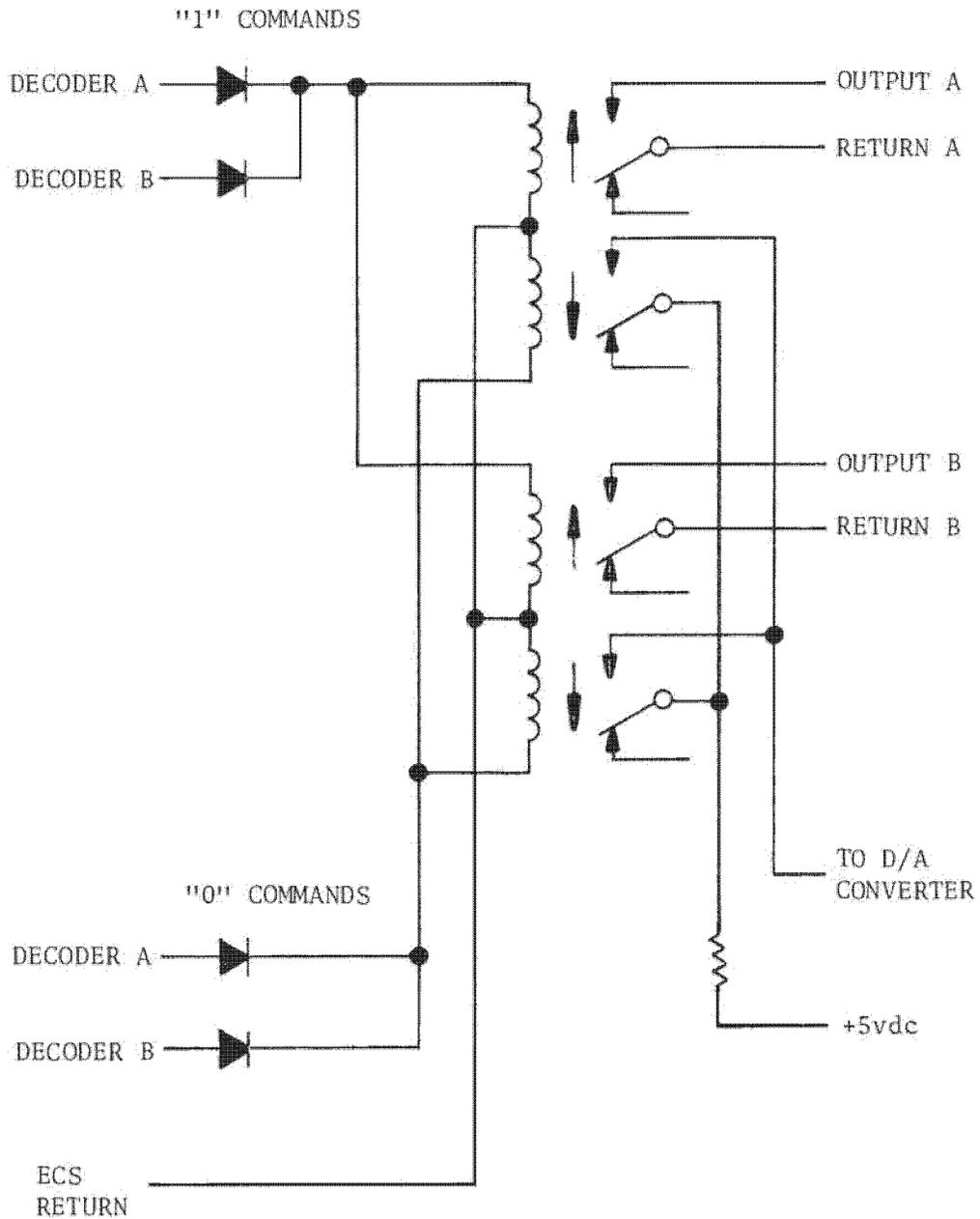
NOTE: Commands may also be coupled through optical isolators, in which case the return line will be the 24.5v power return.
