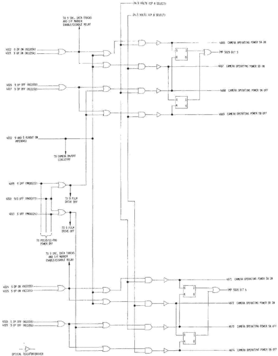
Figure 3.9-24. 9 and 5 Operational Power ON/OFF
