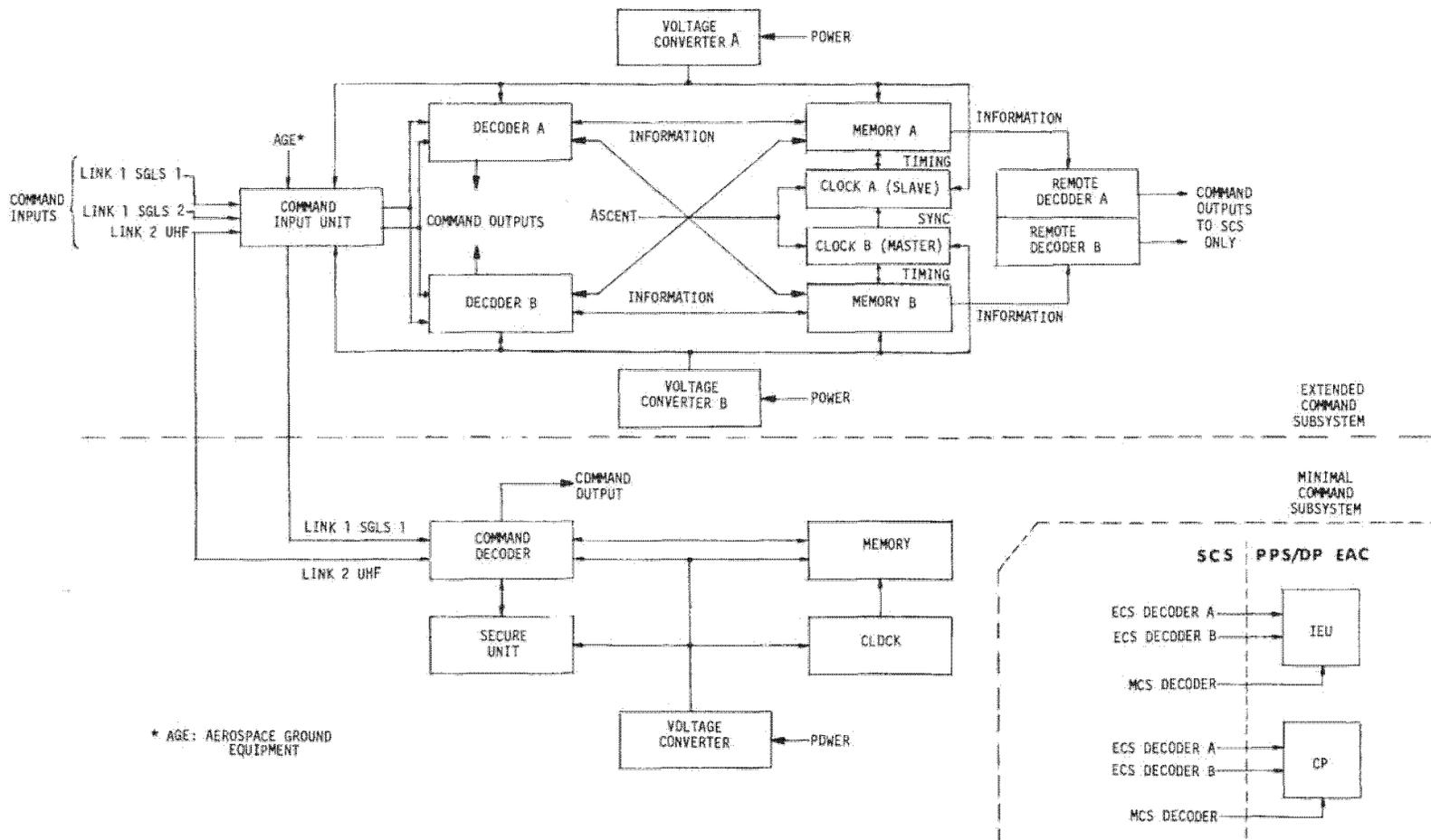
Figure 3.9-1. Command Subsystem Block Diagram
