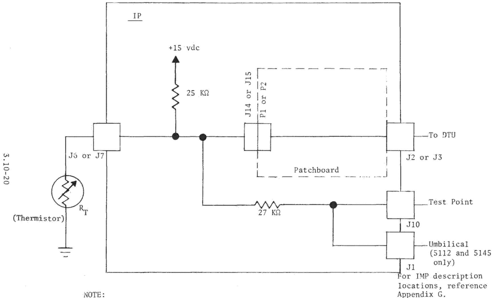
Figure 3.10-9. Typical IP Processing Circuits: IMP's 5111, 5112, and 5145
