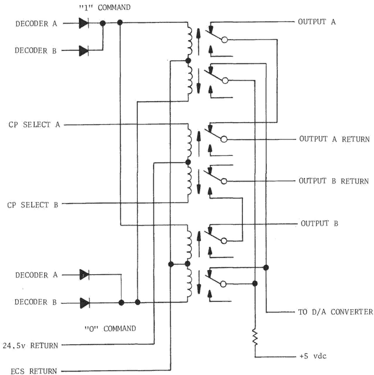
NOTE: Commands may also be coupled through optical isolators, in which case the return will be the 24.5v power return. The basic logic remains unchanged.
