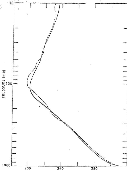
FIGURE 5. DEDUCED TEMPERATURE PROFILE IN CLEAR SKIES FROM DATA IN THE 15-MICRON CARBON DIOXIDE BAND ACQUIRED AT 7:57 A.M. CST BY A BALLOON-BORNE VERSION OF SIRS (SOLID LINE). THE BALLOON WAS LAUNCHED TO AN ALTITUDE OF 100,000 FT. ON SEPTEMBER 11, 1964 FROM PALESTINE, TEXAS. THE DASHED LINE IS THE NOON CST PROFILE FROM THE FORT WORTH RADIOSONDE. (AFTER WARK ET AL., 1967).
