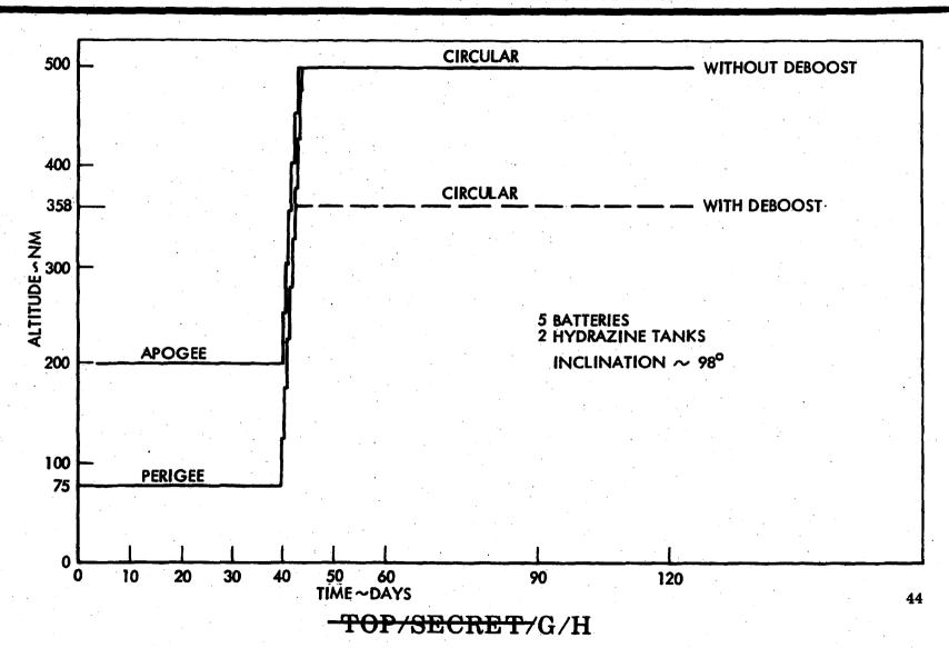
THE INITIAL ORBIT OF A LIKELY DUAL MODE MISSION PROFILE, WITH PERIGEE AND APOGEE AT 75 AND 200 NM RESPECTIVELY, IS AN ORBIT JUST AT THE UPPER END OF THE HISTORICAL RANGE OF GAMBIT MISSIONS. MAINTENANCE OF THIS ORBIT FOR 40 DAYS WOULD CONSUME APPROXIMATELY 32% OF THE AVAILABLE PROPELLANT AND, AT A PHOTOGRAPHIC RATE OF 200 FRAMES PER DAY, WOULD YIELD 8000 FRAMES OF WHICH MORE THAN 70 PERCENT WOULD BE EXPECTED TO BE CLOUD FREE.
