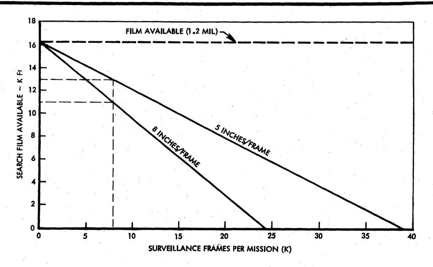
UTILIZING A FILM WITH A BASE THICKNESS OF 1.2 MILS, THE CURRENT GAMBIT VEHICLE HAS A FILM SUPPLY OF 12,600 FT OF 9-INCH FILM AND 3,600 FT OF 5-INCH FILM FOR A COMBINED TOTAL OF 16,200 FT. THIS FILM MAY BE USED IN THE CURRENT GAMBIT MODE AT LOW ALTITUDE FOR HIGH RESOLUTION SURVEILLANCE, OR ALTERNATIVELY, AT HIGH ALTITUDE FOR SEARCH.
