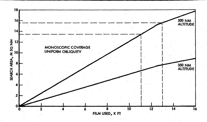
THE INCREASED SCALE AT HIGHER ALTITUDES PROVIDES THE GAMBIT SATELLITE WITH THE CAPABILITY OF PHOTOGRAPHING A SIGNIFICANT AREA. THE MONOSCOPIC AREA COVERAGE CAPABILITY OF A SINGLE VEHICLE IS SHOWN IN THE FACING FIGURE AS A FUNCTION OF FILM USAGE AT EITHER OF TWO ALTITUDES, 350 AND 500 NM. THE BREAKS IN THE SLOPES OF THE LINES OCCUR AS THE 9-INCH FILM SUPPLY IS EXHAUSTED AT 12,600 FT AND CONTINUES UNTIL THE 5-INCH FILM IS EXPENDED AT 16,200 FT.
