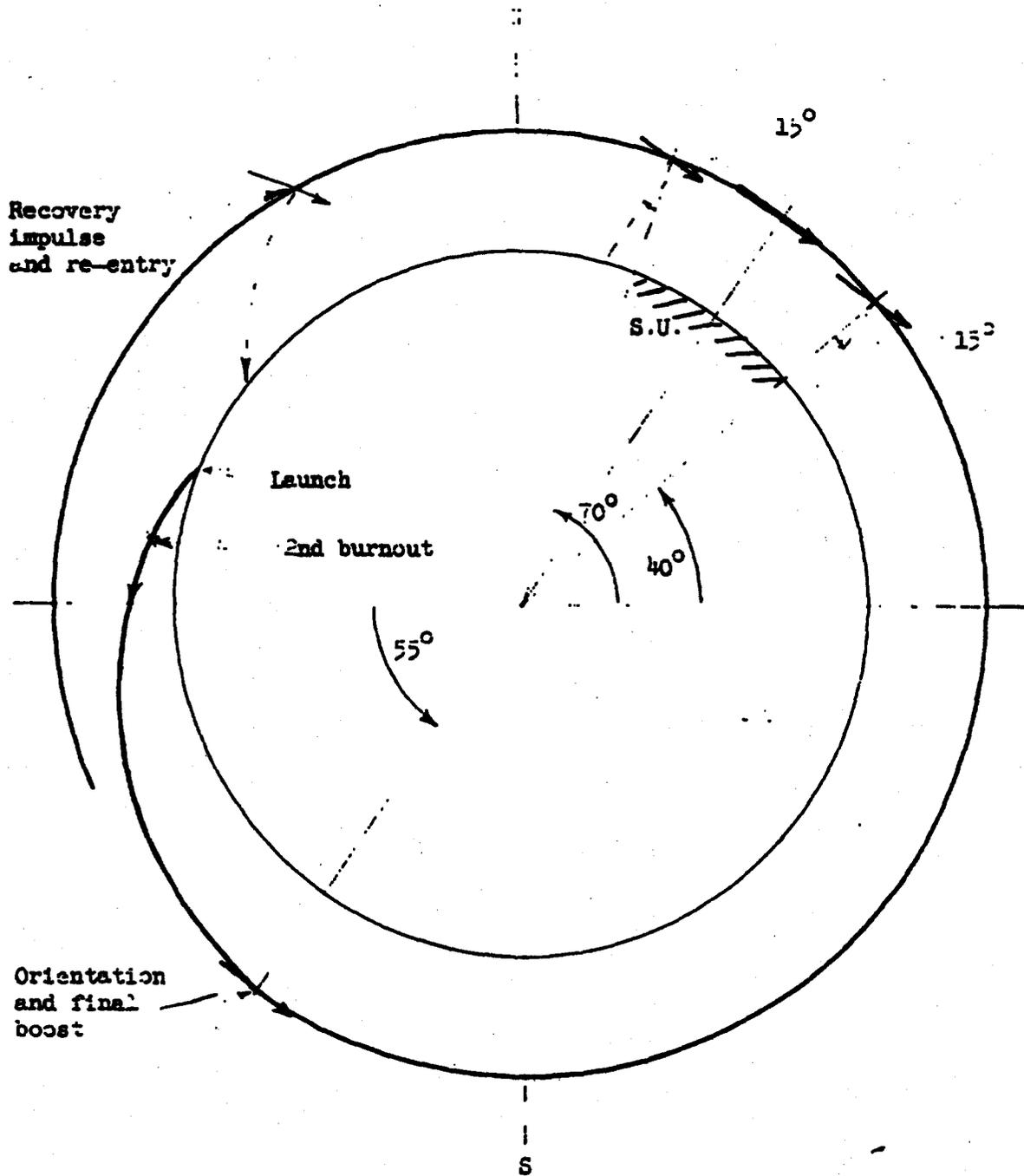
Fig. 2 Trajectory and Payload Attitude
