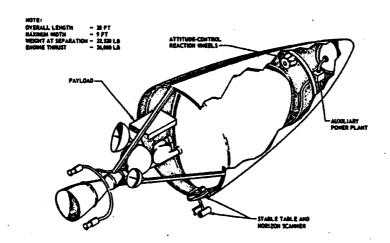
Fig. 1 Satellite Vehicle Proposed by RAND, 1954
