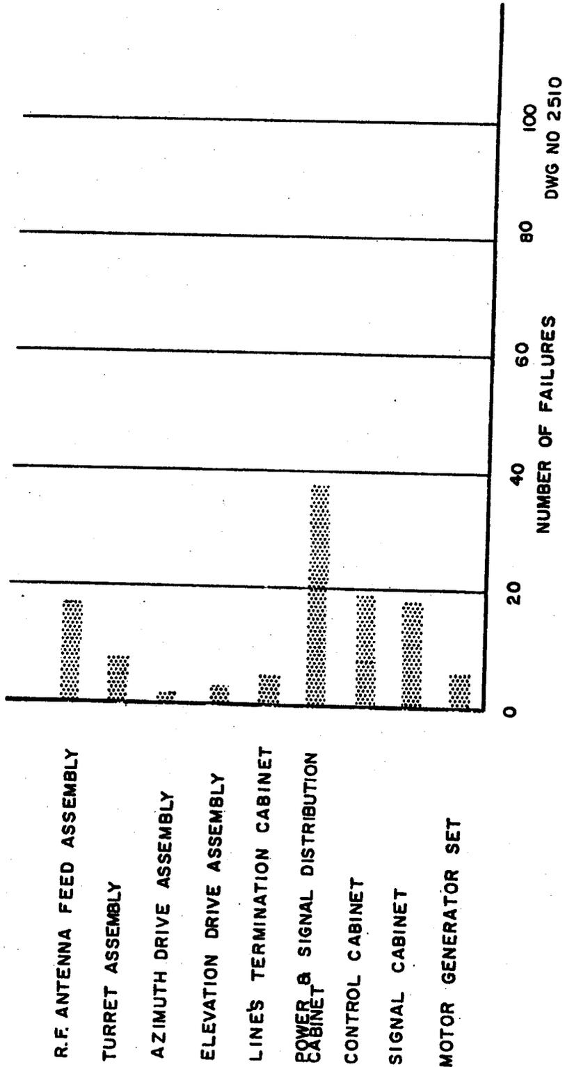
Fig. 9-5 Telemetry Tracker (R-1162) Component Failures
