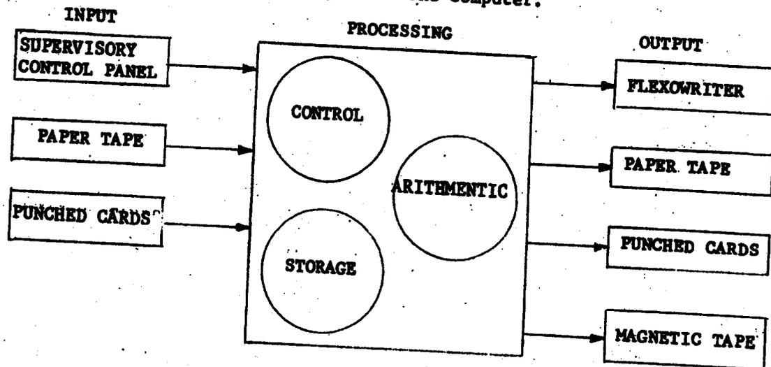
Figure 6-1 1103-AF Automatic Digital Computer System
