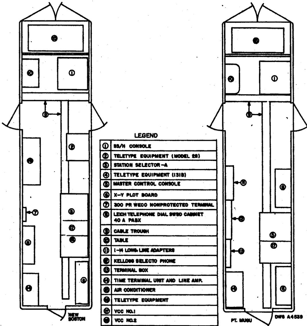
Fig. 4-9 Administration and Control Van, Floor Plan
