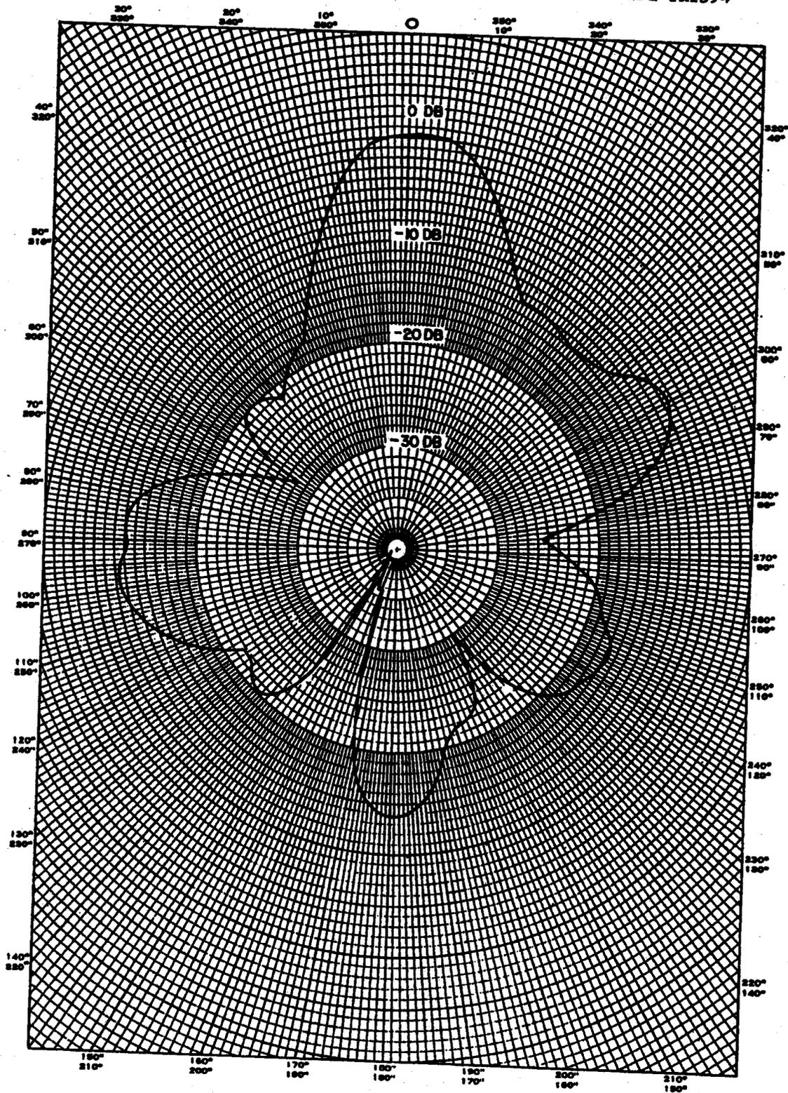
Fig. 3-8 Tri-Helix Antenna Horizontal Directivity Pattern
