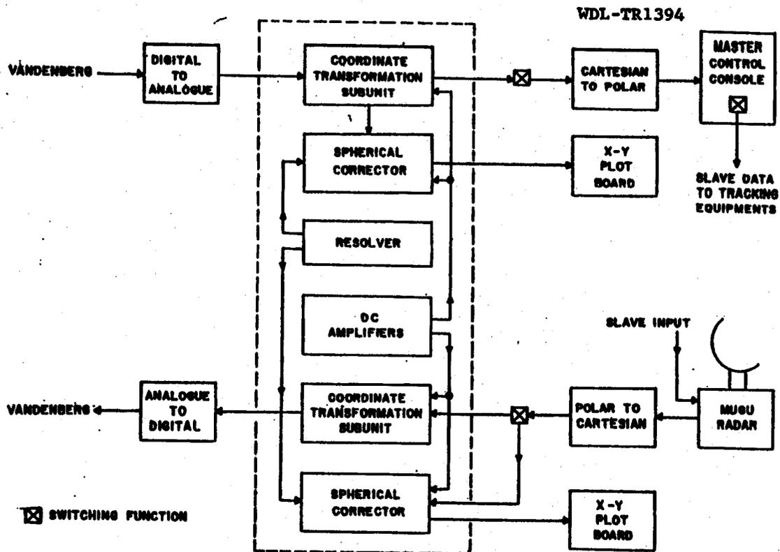
Fig. 4-24 Coordinate Transformation Unit Block Diagram
