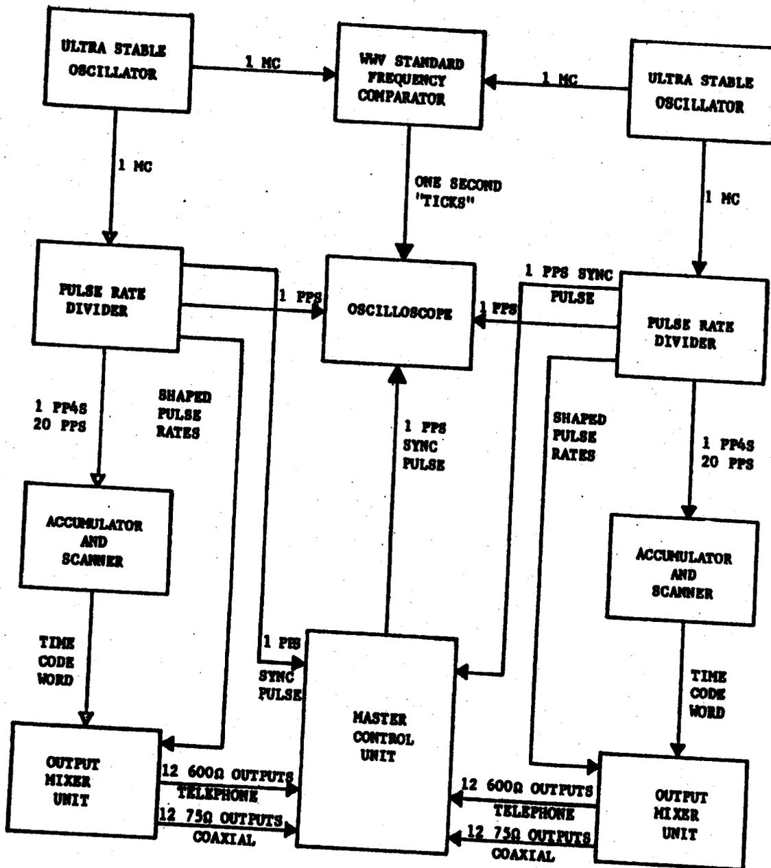
Fig. 5-3 Central Dual Timing Generator Block Diagram
