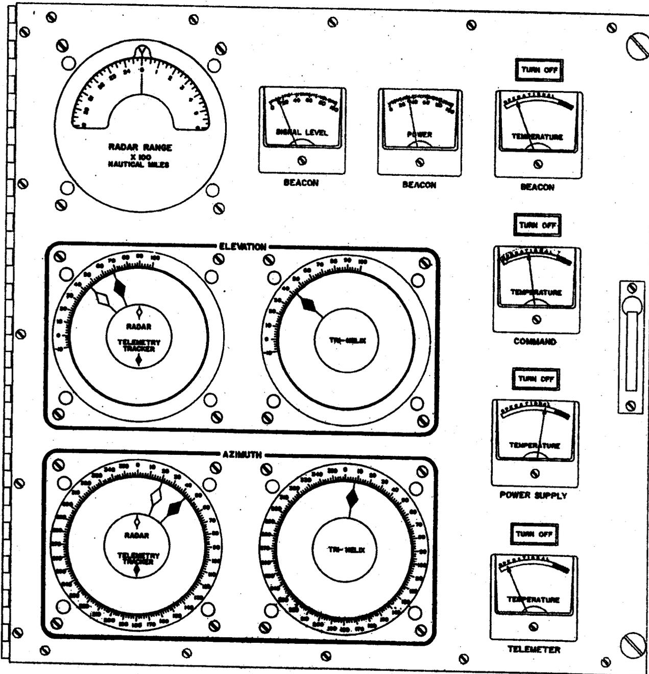
Fig. 4-40 Tracking Indicator Panel
