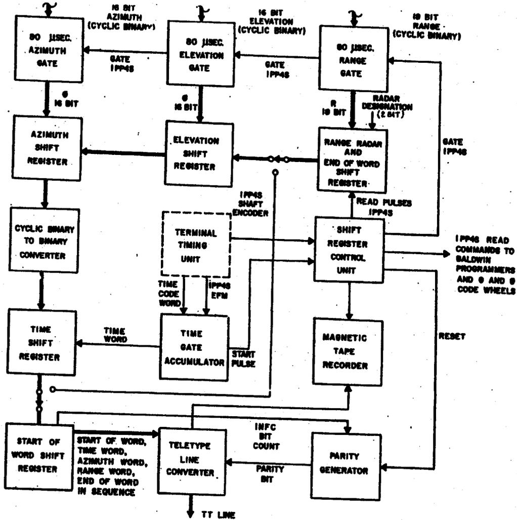
Fig. 4-12 Digital/Teletype Converter Block Diagram
