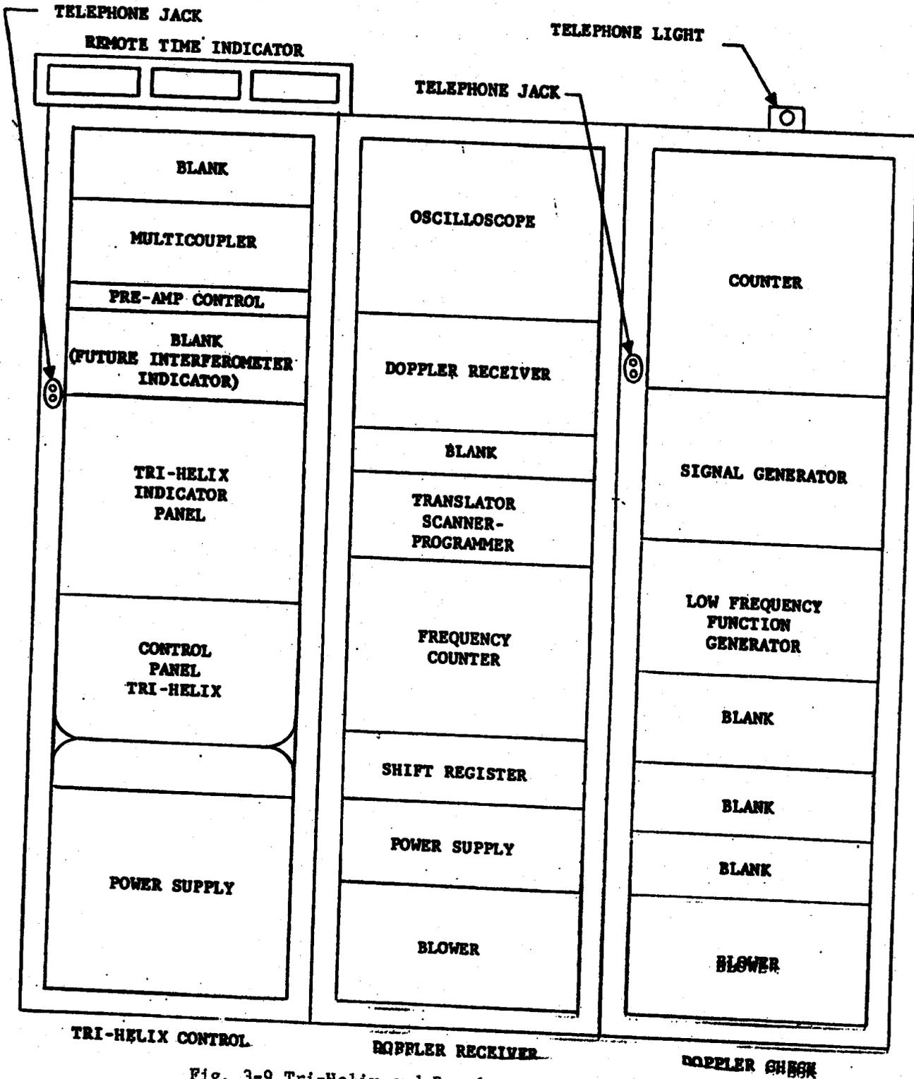
Fig. 3-9 Tri-Helix and Doppler Control Rack Layout
