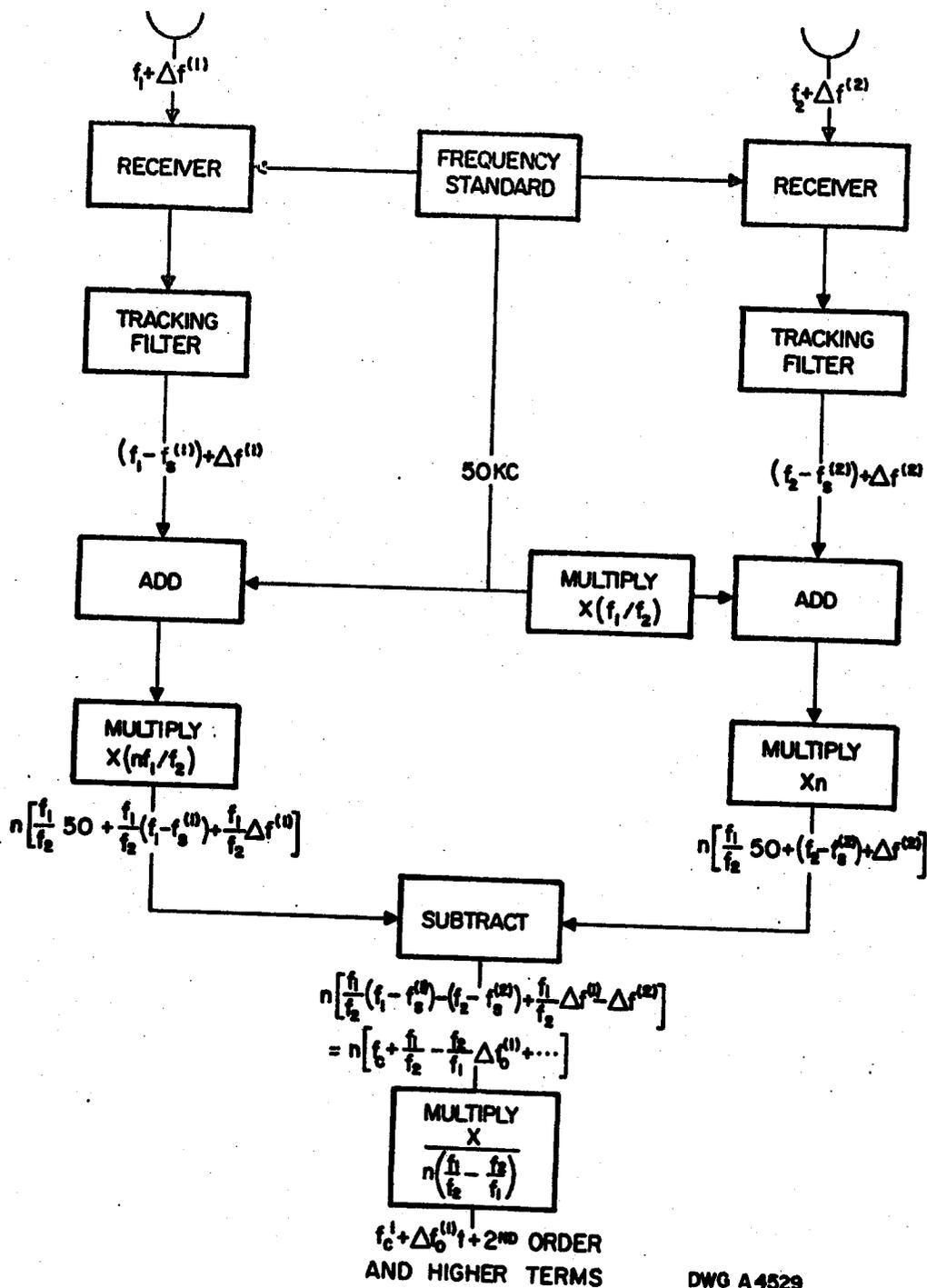
Fig. 3-19 Analog Refraction Correction Unit
