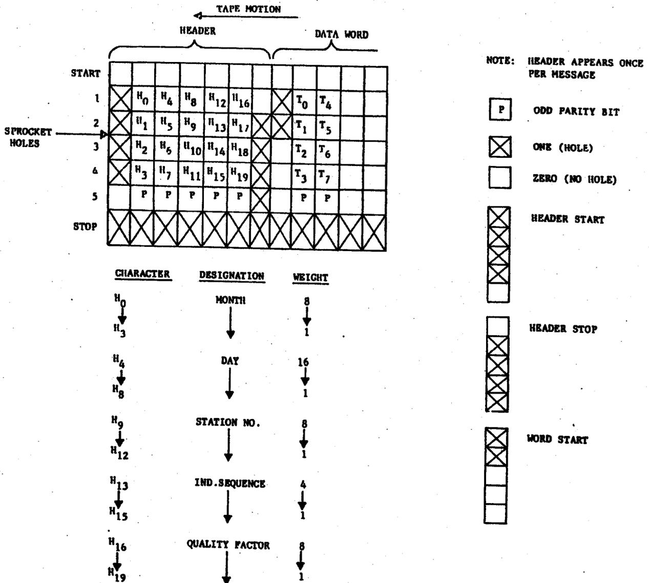
Fig. 6-2 Typical Header Teletype Format to Central Computer
