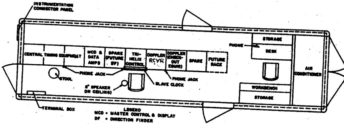
Fig. 3-10 Typical Instrumentation Van Floor Plan
