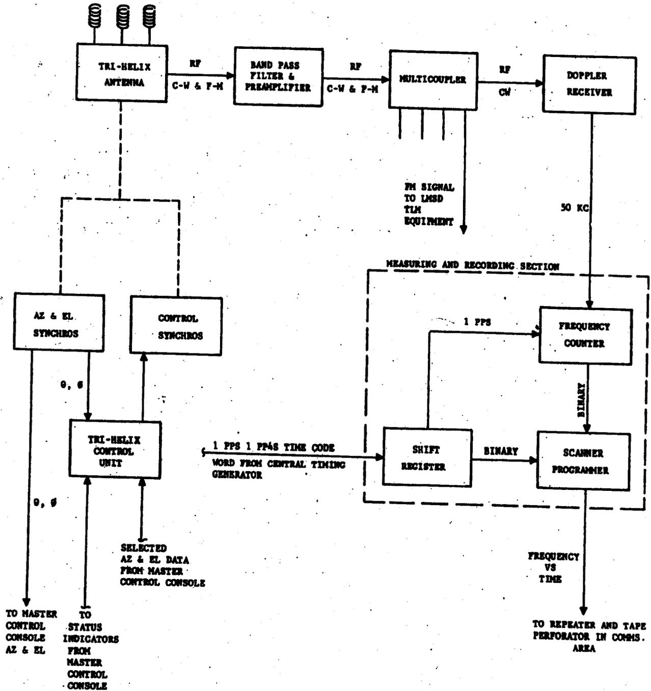
Fig. 3-6 Doppler System Block Diagram
