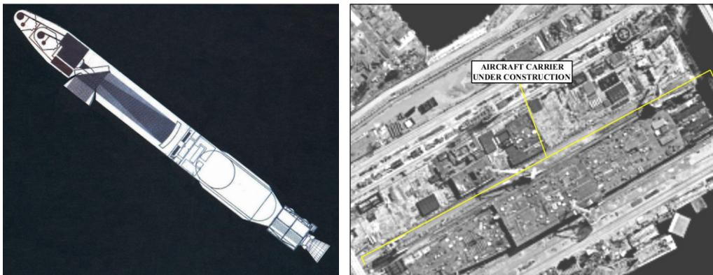
Figure 3a (left). Schematic of Gambit-3 spacecraft (28.6 ft long, 5 feet diameter). Figure 3b (right). Gambit image of a Soviet aircraft carrier under construction at Mykolayiv, 4 July 1984. (Photos courtesy of CSNR Reference Collection.)
