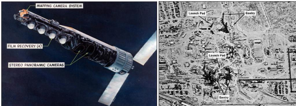
Figure 4a (left). Artist Concept of Hexagon Vehicle (60 ft long, diameter 10 ft). Figure 4b (right). Hexagon Panoramic photograph of Tyuratam Missile Test Range in Former USSR, August 1984.<sup>14</sup> (Photos courtesy, CSNR Reference Collection.)
