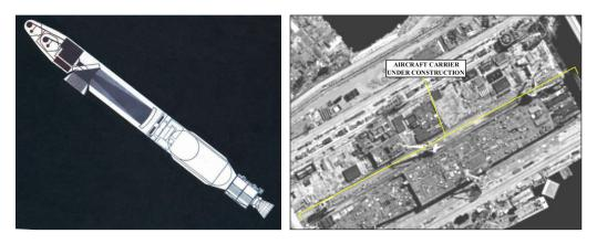
Figure 3a (left). Schematic of Gambit-3 spacecraft (28.6 ft long, 5 feet diameter). Figure 3b (right). Gambit image of a Soviet aircraft carrier under construction at Mykolayiv, 4 July 1984. (Photos courtesy of CSNR Reference Collection.)
