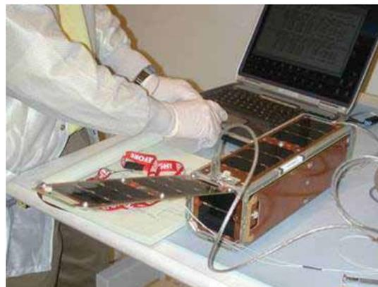
*(U) Weather Colony Program CubeSats undergoing Payload Accommodation Study at the Naval Research Laboratory to determine candidate configurations for placing space weather sensors on a CubeSat.*
