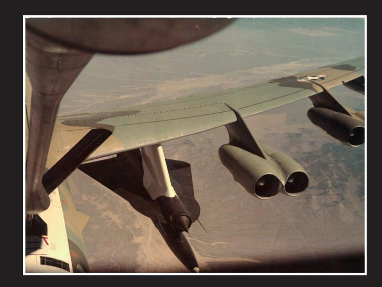
D-21 drone under B-52 wing during inflight refueling. (
