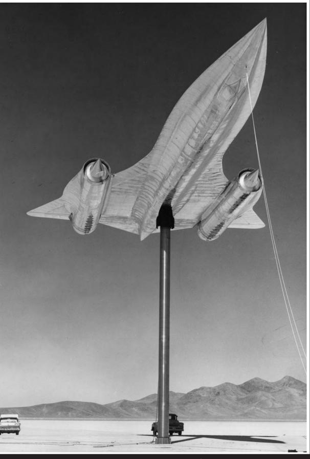
A-12 aircraft mock-up undergoing radar testing. ◀
