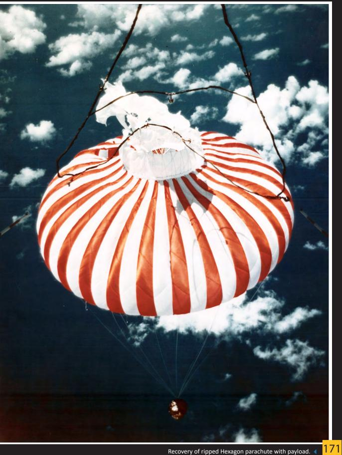
Hexagon Mark VIII recovery parachute and film canister.
